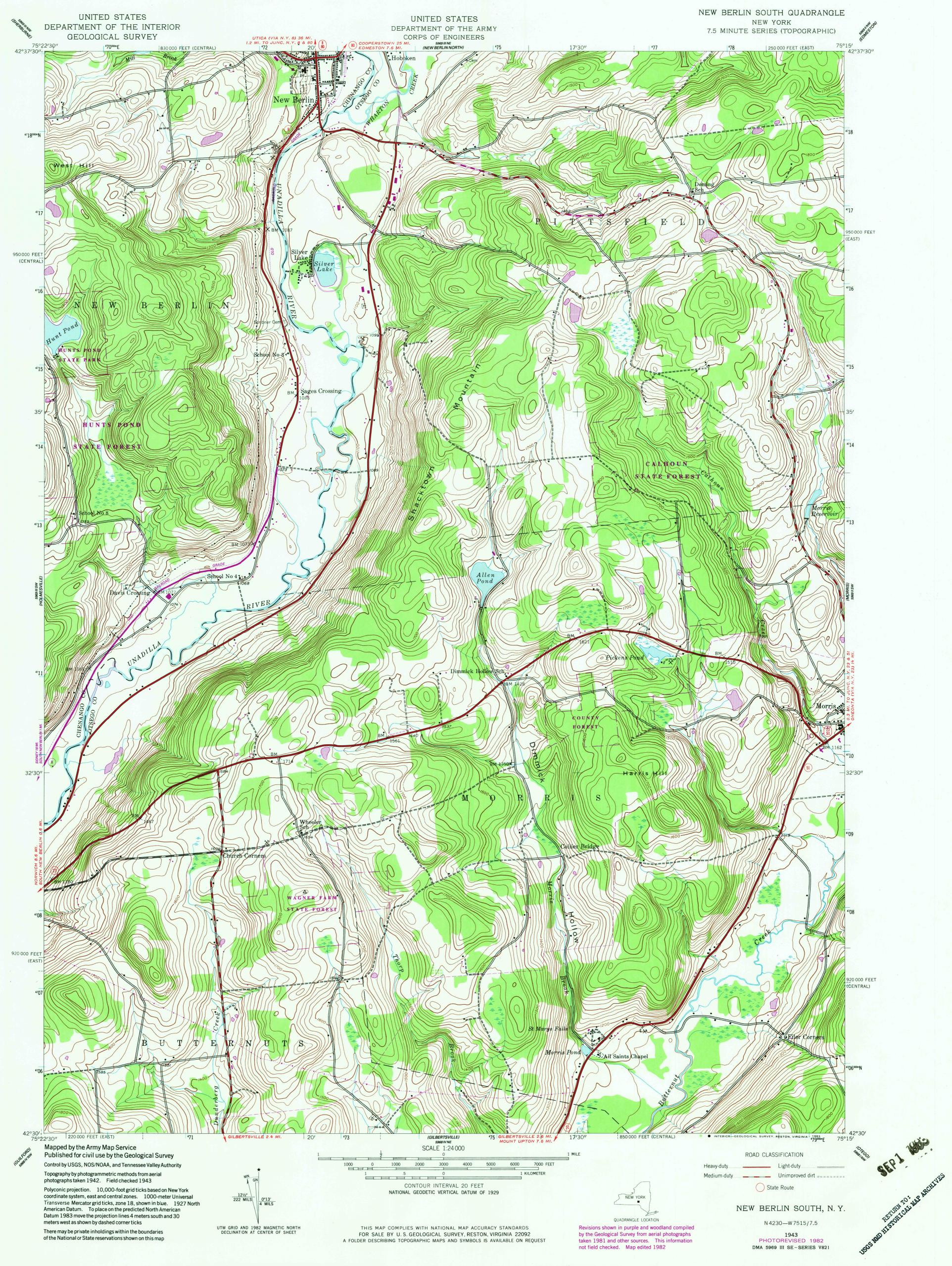
Polyconic projection. 10,000-foot grid ticks based on New York coordinate system, east and central zones. 1000-meter Universal Transverse Mercator grid ticks, zone 18, shown in blue. 1927 North American Datum. To place on the predicted North American Datum 1983 move the projection lines 4 meters south and 30 meters west as shown by dashed corner ticks
