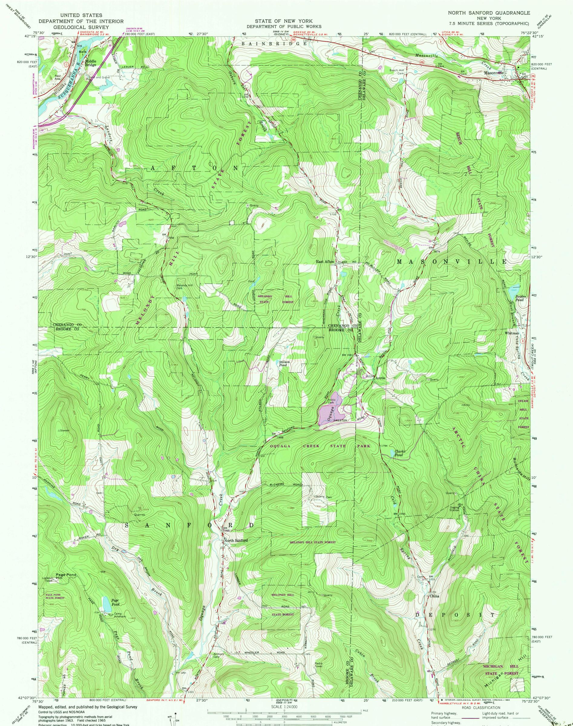
Polyconic projection. 10,000-foot grid ticks based on New York coordinate system, central and east zones. 1000-meter Universal Transverse Mercator grid ticks, zone 18, shown in blue 1927 North American Datum. To place on the predicted North American Datum 1983 move the projection lines 4 meters south and 30 meters west as shown by dashed corner ticks
