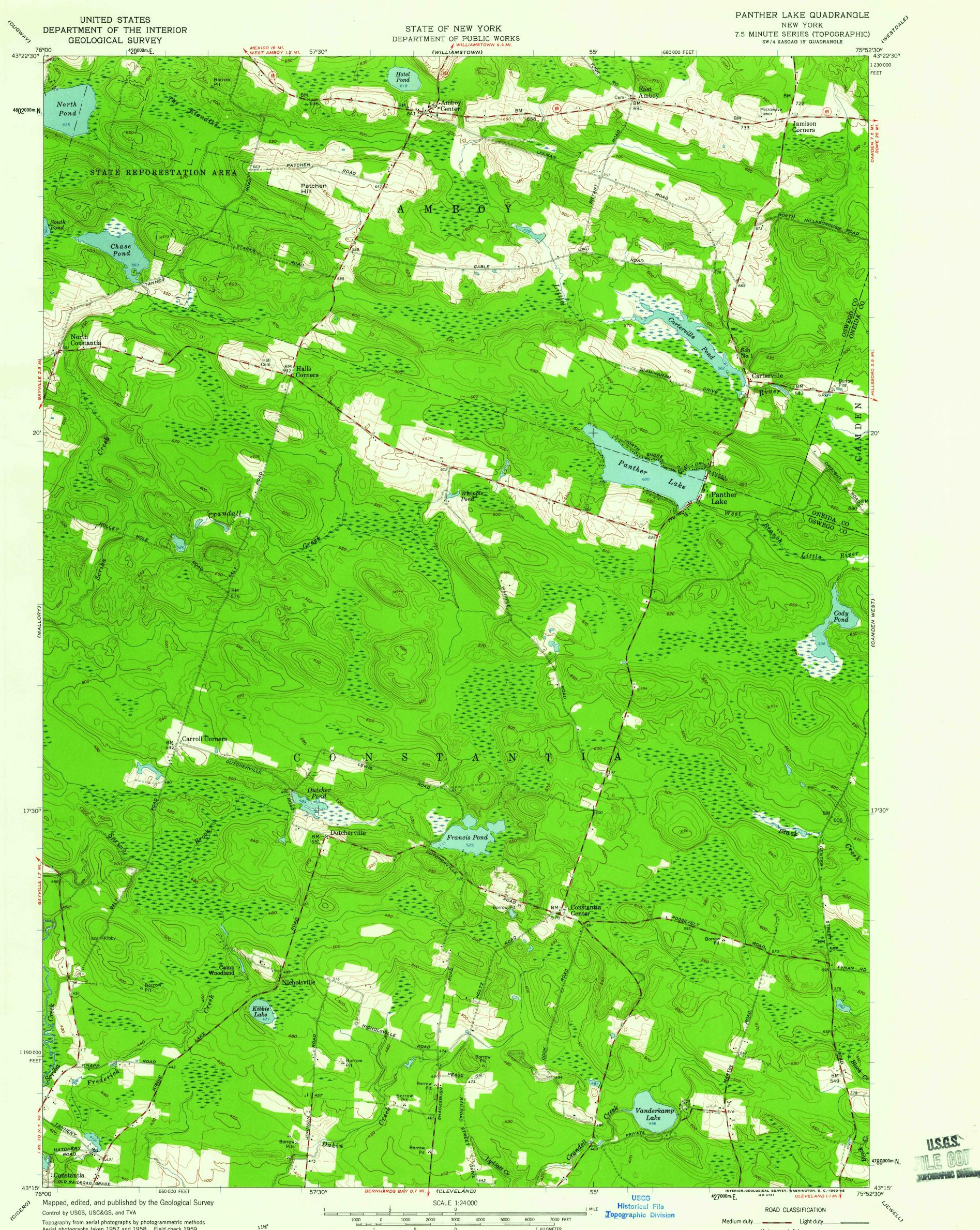
Aerial photographs taken 1957 and 1958. Field check 1959 Polyconic projection. 1927 North American datum 10,000-foot grid based on New York coordinate system, central zone 1000-meter Universal Transverse Mercator grid ticks, zone 18, shown in blue Fine red dashed lines indicate selected fence and field lines visible on aerial photographs. This information is unchecked
