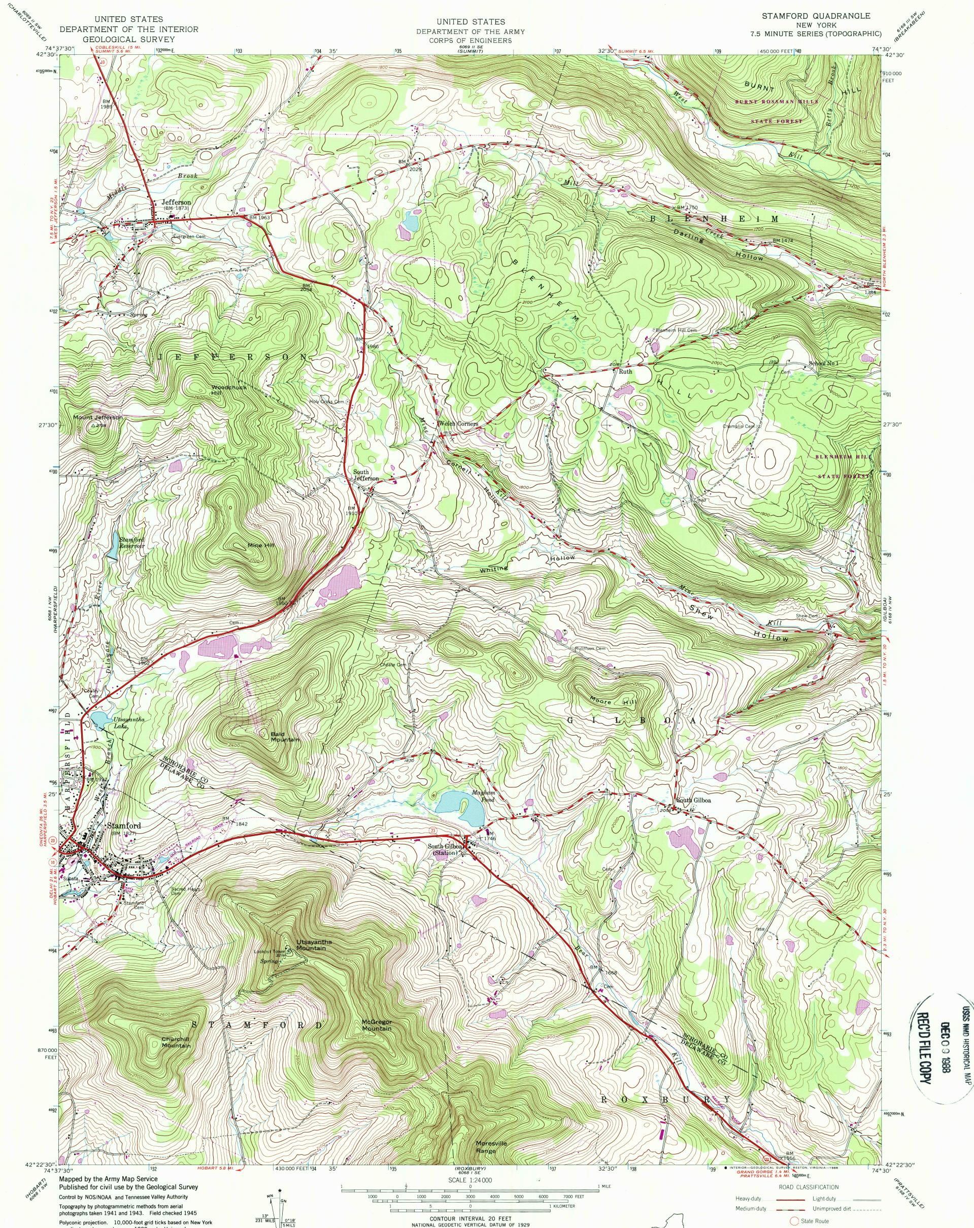
Polyconic projection. 10,000-foot grid ticks based on New York coordinate system, east zone. 1000-meter Universal Transverse Mercator grid ticks, zone 18, shown in blue 1927 North American Datum. To place on the predicted North American Datum 1983 move the projection lines 5 meters south and 33 meters west as shown by dashed corner ticks
