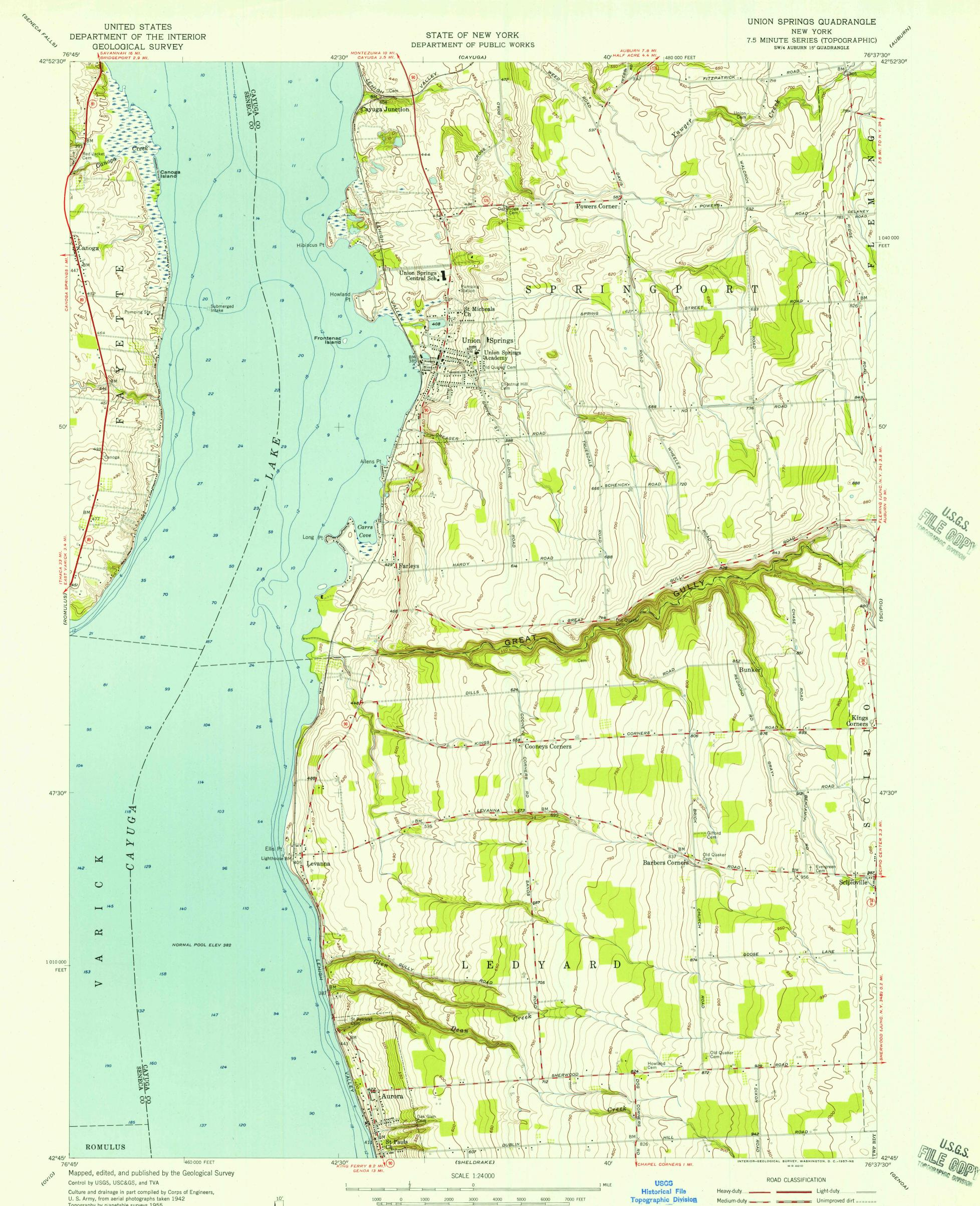
Topography by planetable surveys 1955 Hydrography from U. S. Lake Survey chart 187, (1952) Polyconic projection. 1927 North American datum 10,000-foot grid based on New York coordinate system, central zone
