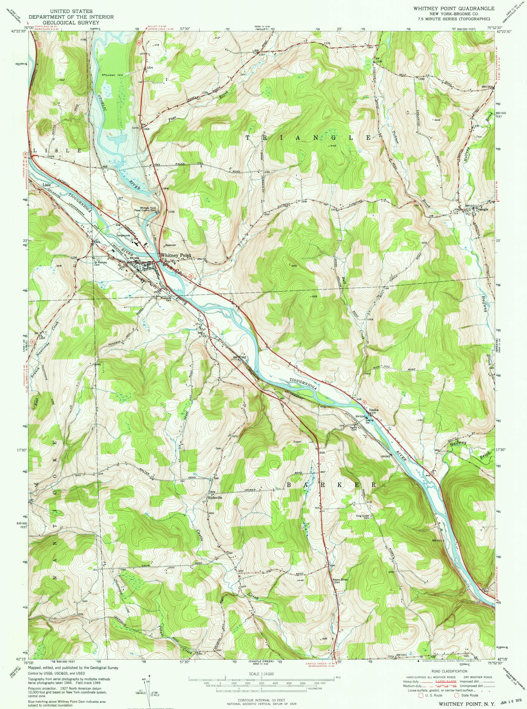
Blue hatching above Whitney Point Dam indicates area subject to controlled inundation UTM GRID AND 1949 MAGNETIC NORTH DECLINATION AT CENTER OF SHEET 1000-metre Universal Transverse Mercator grid ticks, zone 18, shown in blue
