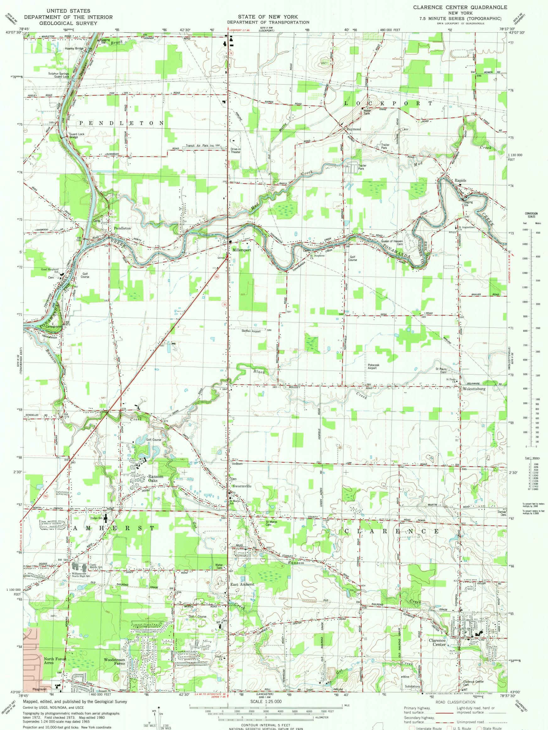
Projection and 10,000-foot grid ticks: New York coordinate system, west zone (transverse Mercator) 1000-meter Universal Transverse Mercator grid, zone 17 1927 North American Datum To place on the predicted North American Datum 1983 UTM GRID AND 1980 MAGNETIC NORTH DECLINATION AT CENTER OF SHEET move the projection lines 2 meters south and 20 meters west as shown by dashed corner ticks
