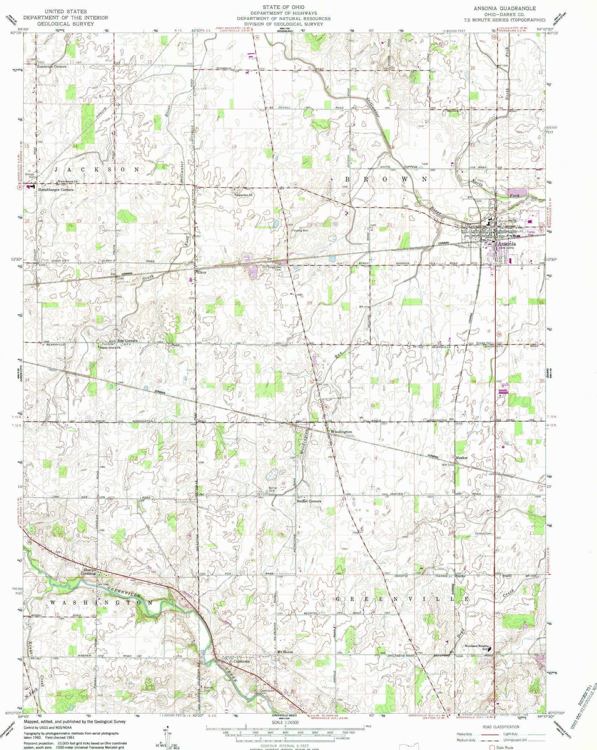
system, south zone. 1000-meter Universal Transverse Mercator grid ticks, zone 16, shown in blue. 1927 North American Datum To place on the predicted North American Datum 1983 move the projection lines 2 meters south and 4 meters west as shown by dashed corner ticks
