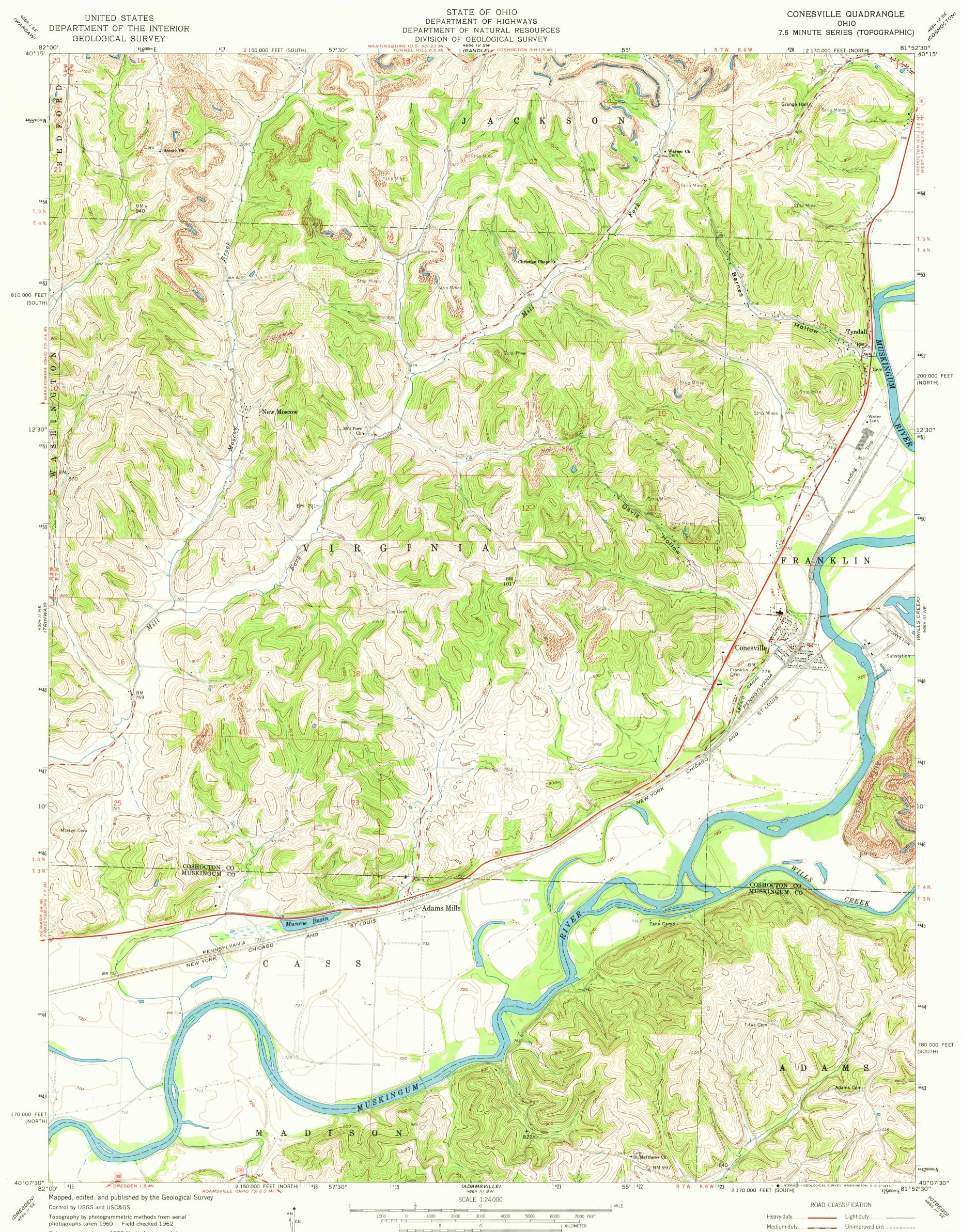
Polyconic projection. 1927 North American datum 10,000-foot grids based on Ohio coordinate system, north and south zones 1000-meter Universal Transverse Mercator grid ticks, zone 17, shown in blue
