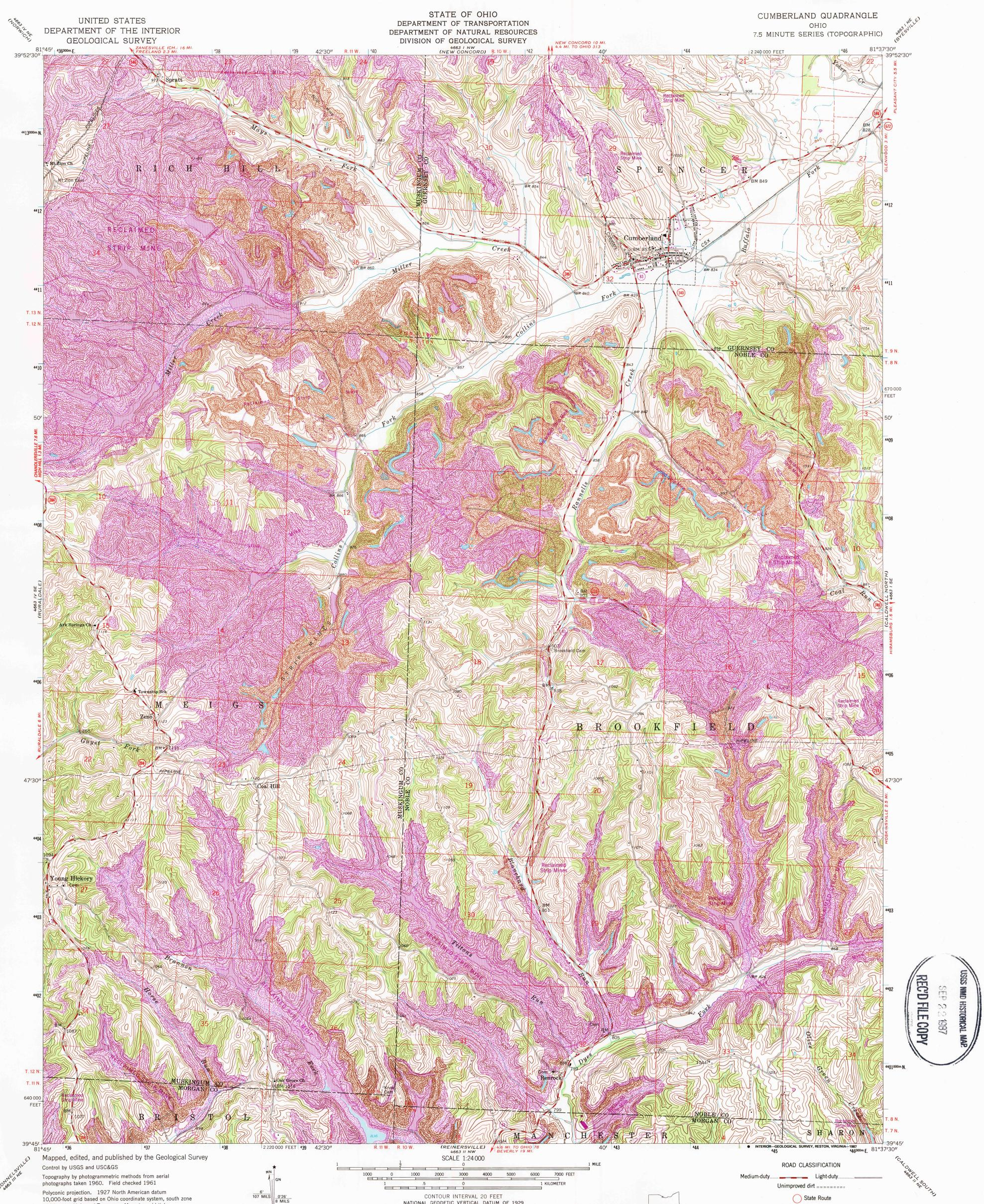
Polyconic projection. 1927 North American datum 10,000-foot grid based on Ohio coordinate system, south zone 1000-meter Universal Transverse Mercator grid ticks, zone 17, shown in blue
