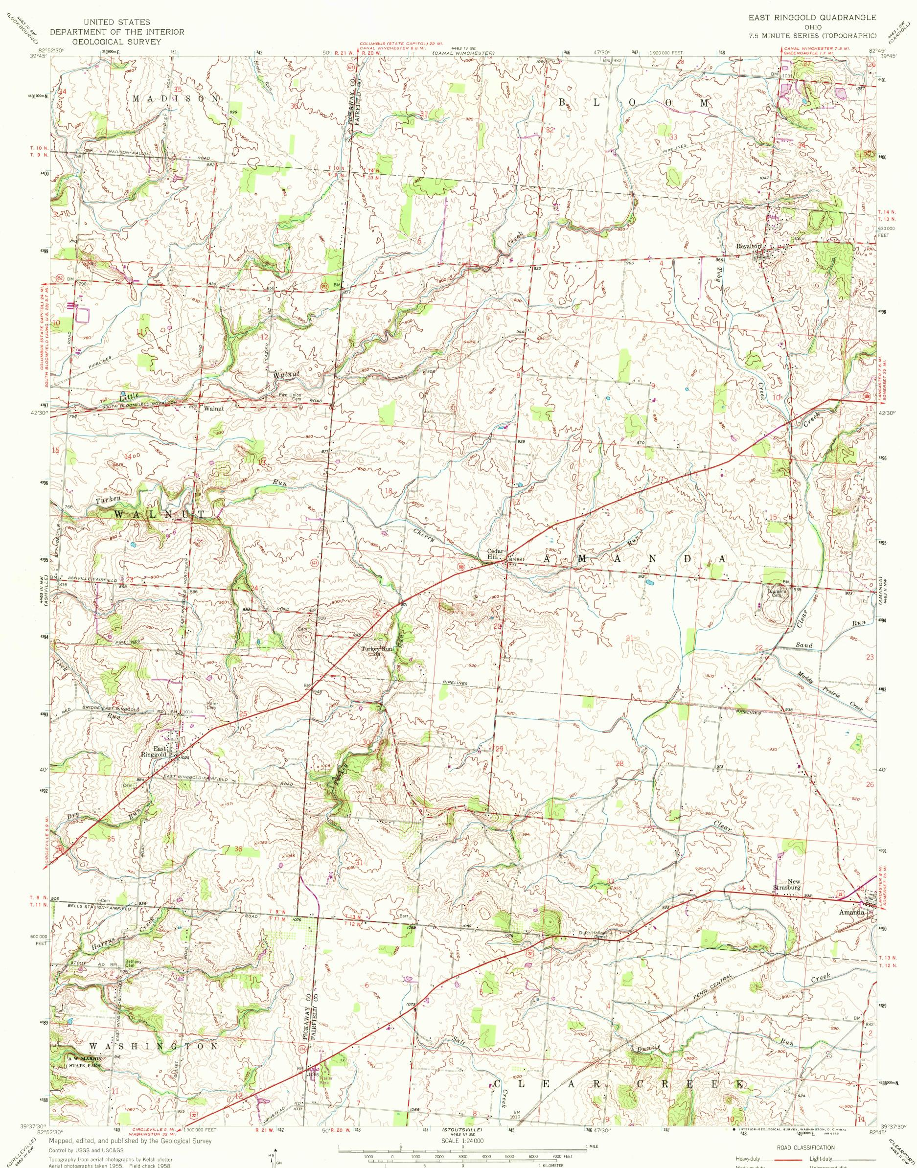
Aerial photographs taken 1955. Field check 1958 Polyconic projection. 1927 North American datum 10,000-foot grid based on Ohio coordinate system, south zone 1000-meter Universal Transverse Mercator grid ticks, zone 17, shown in blue
