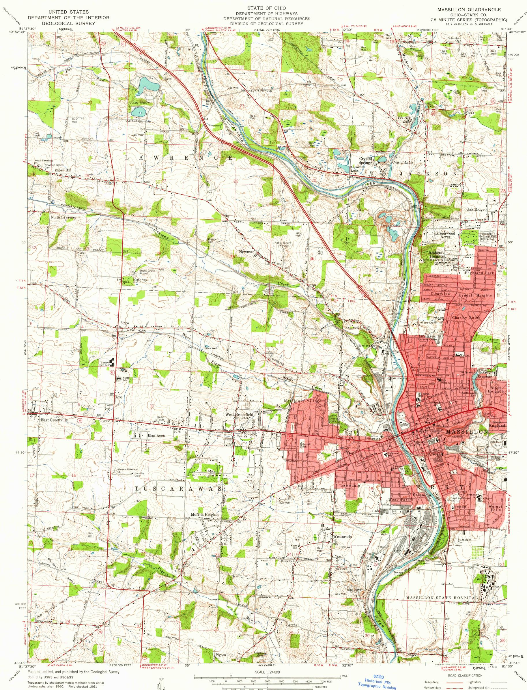
Polyconic projection. 1927 North American datum 10,000-foot grid based on Ohio coordinate system, north zone 1000-meter Universal Transverse Mercator grid ticks, zone 17, shown in blue
