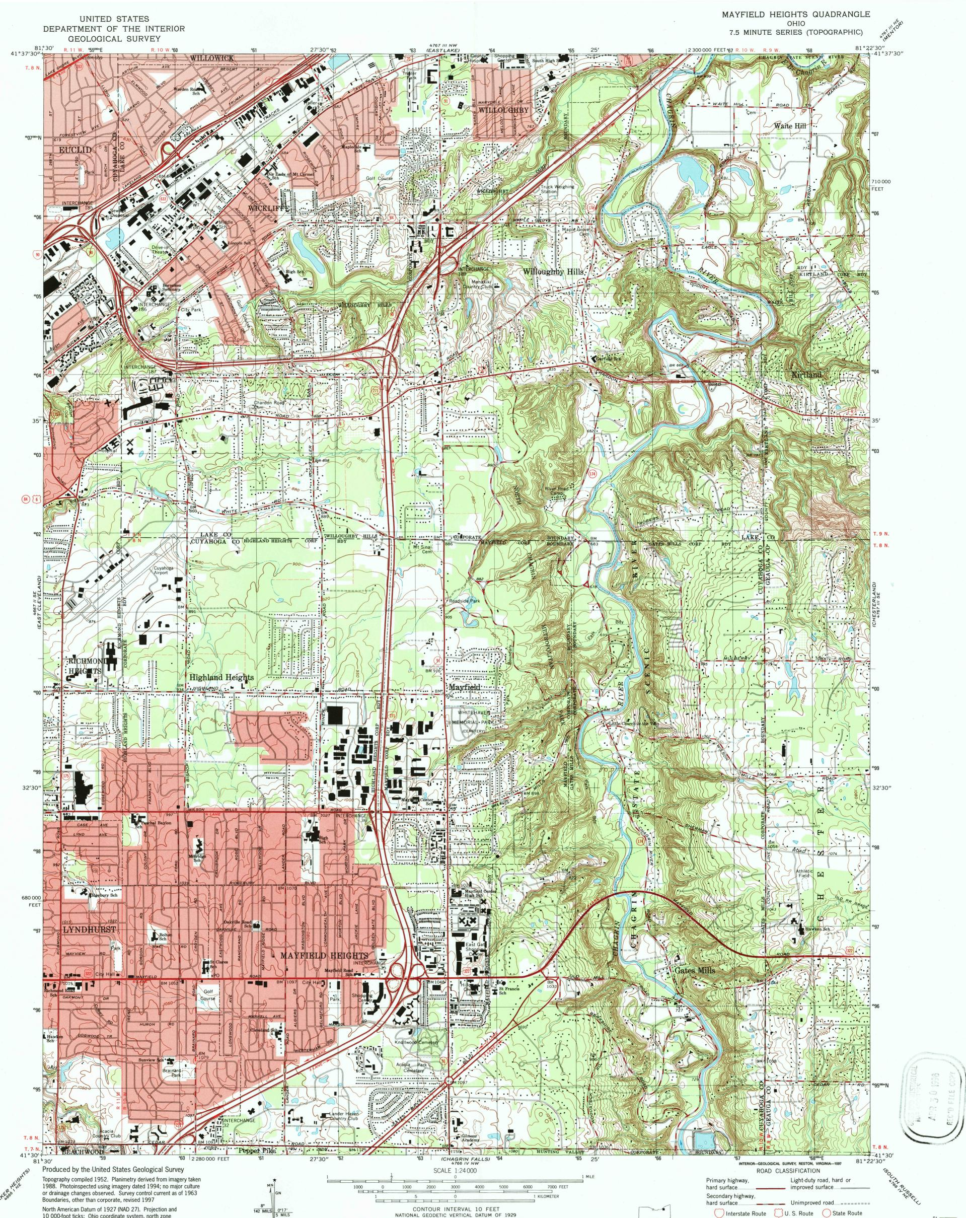
North American Datum of 1927 (NAD 27). Projection and 10 000-foot ticks: Ohio coordinate system, north zone (Lambert conformal conic) 1000-meter Universal Transverse Mercator grid, zone 17
