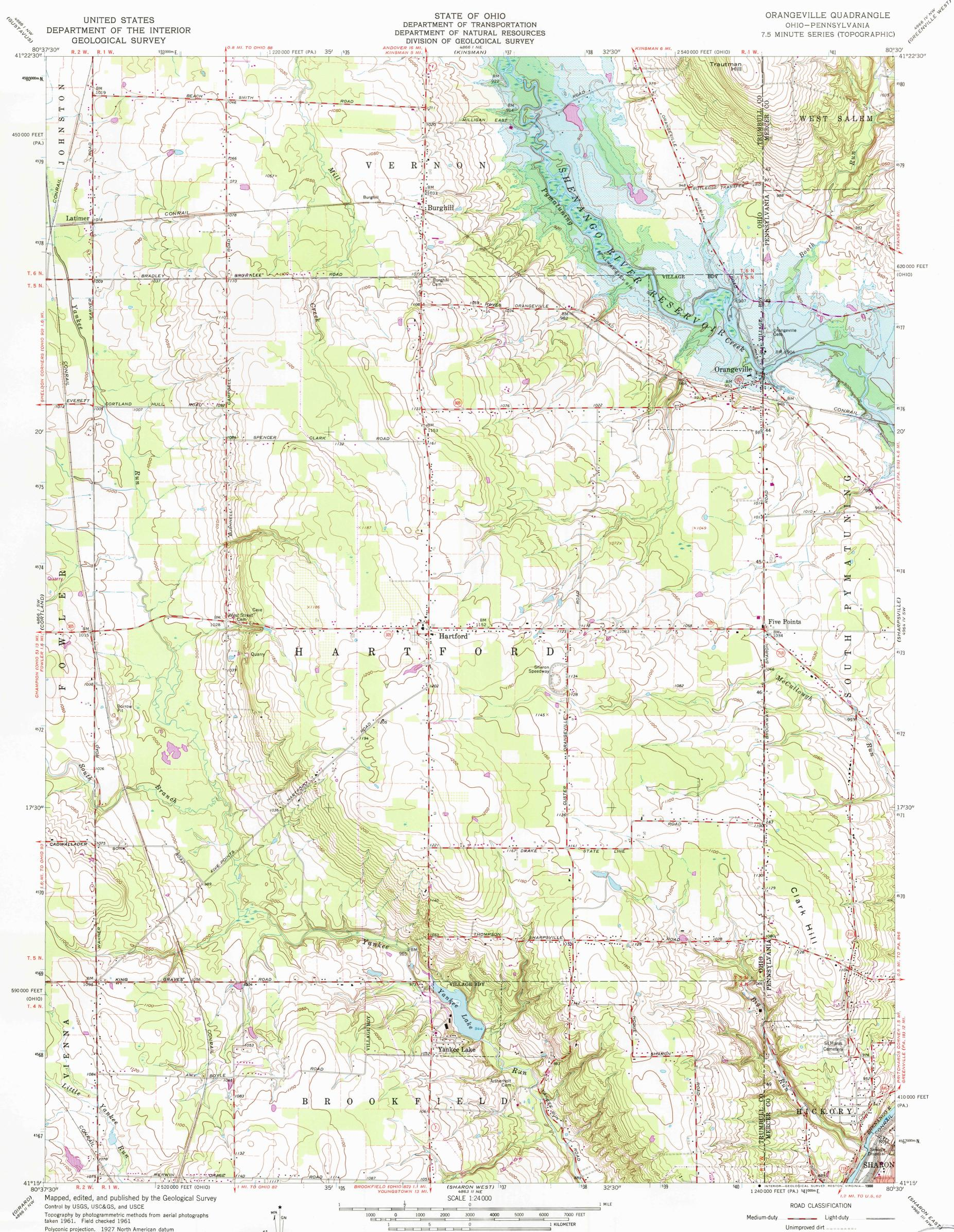
10,000-foot grids based on Ohio coordinate system, north zone and Pennsylvania coordinate system, north zone 1000-meter Universal Transverse Mercator grid ticks, zone 17, shown in blue
