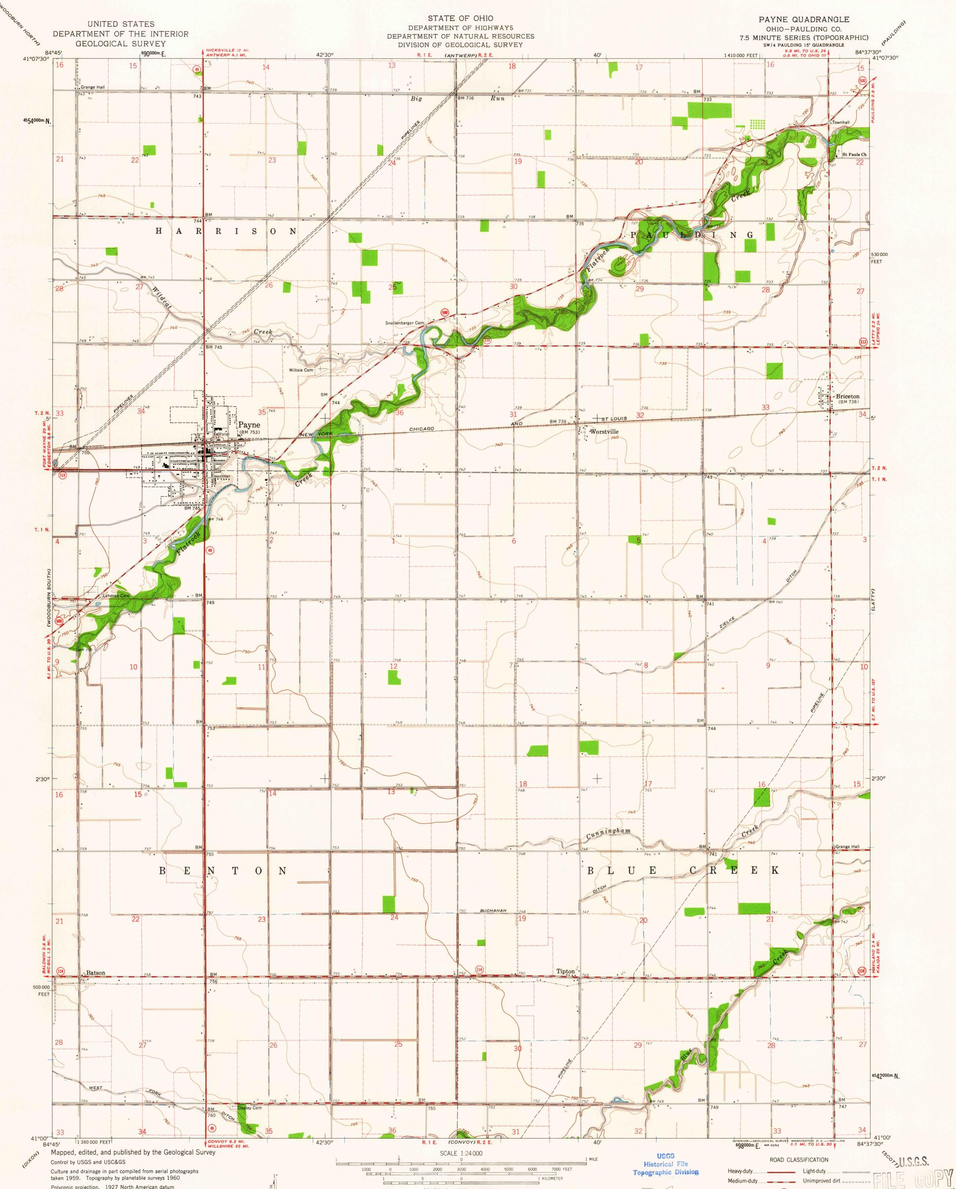
Polyconic projection. 1927 North American datum 10,000-foot grid based on Ohio coordinate system, north zone 1000-meter Universal Transverse Mercator grid ticks, zone 16, shown in blue
