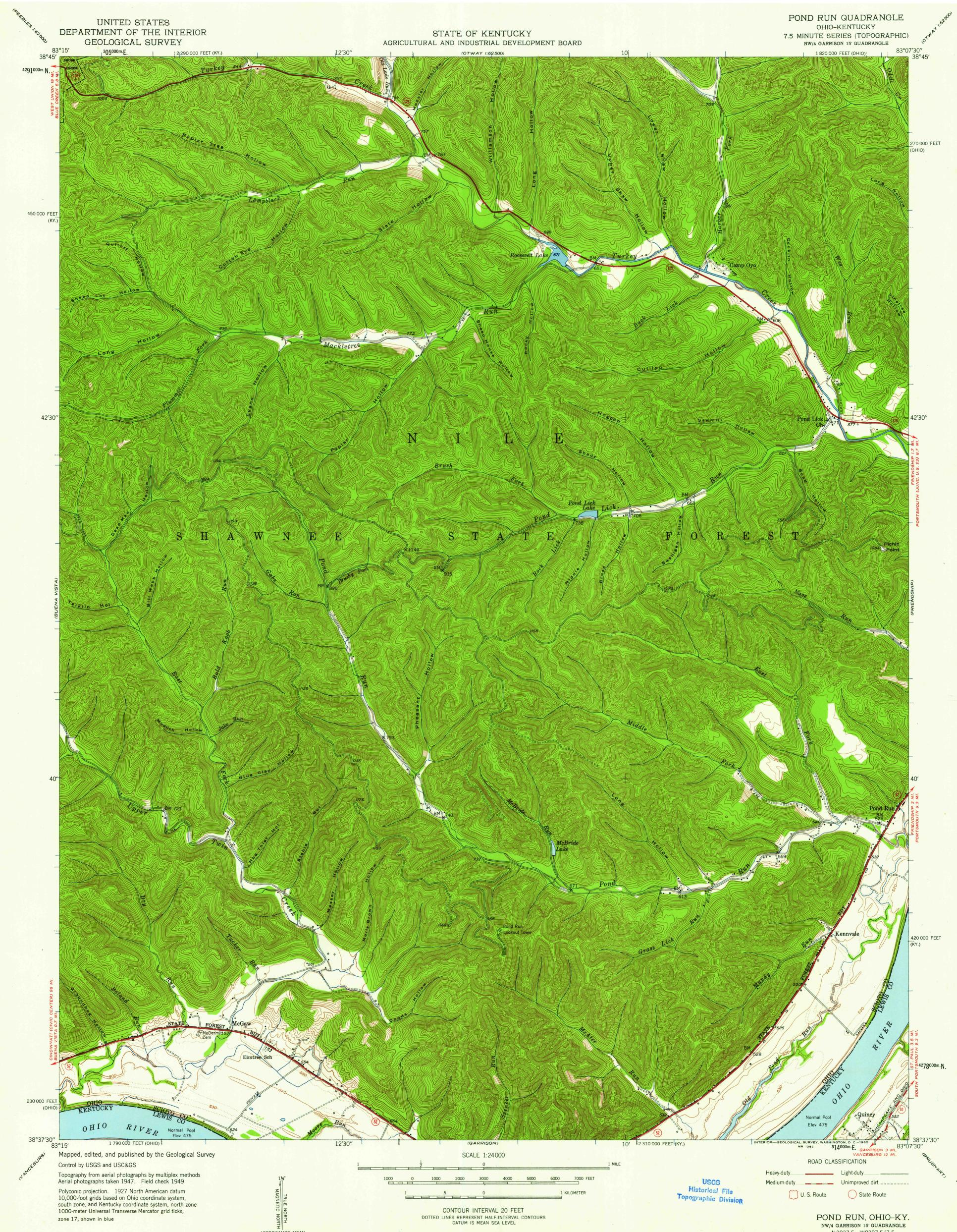
Polyconic projection. 1927 North American datum 10,000-foot grids based on Ohio coordinate system, south zone, and Kentucky coordinate system, north zone 1000-meter Universal Transverse Mercator grid ticks, zone 17, shown in blue
