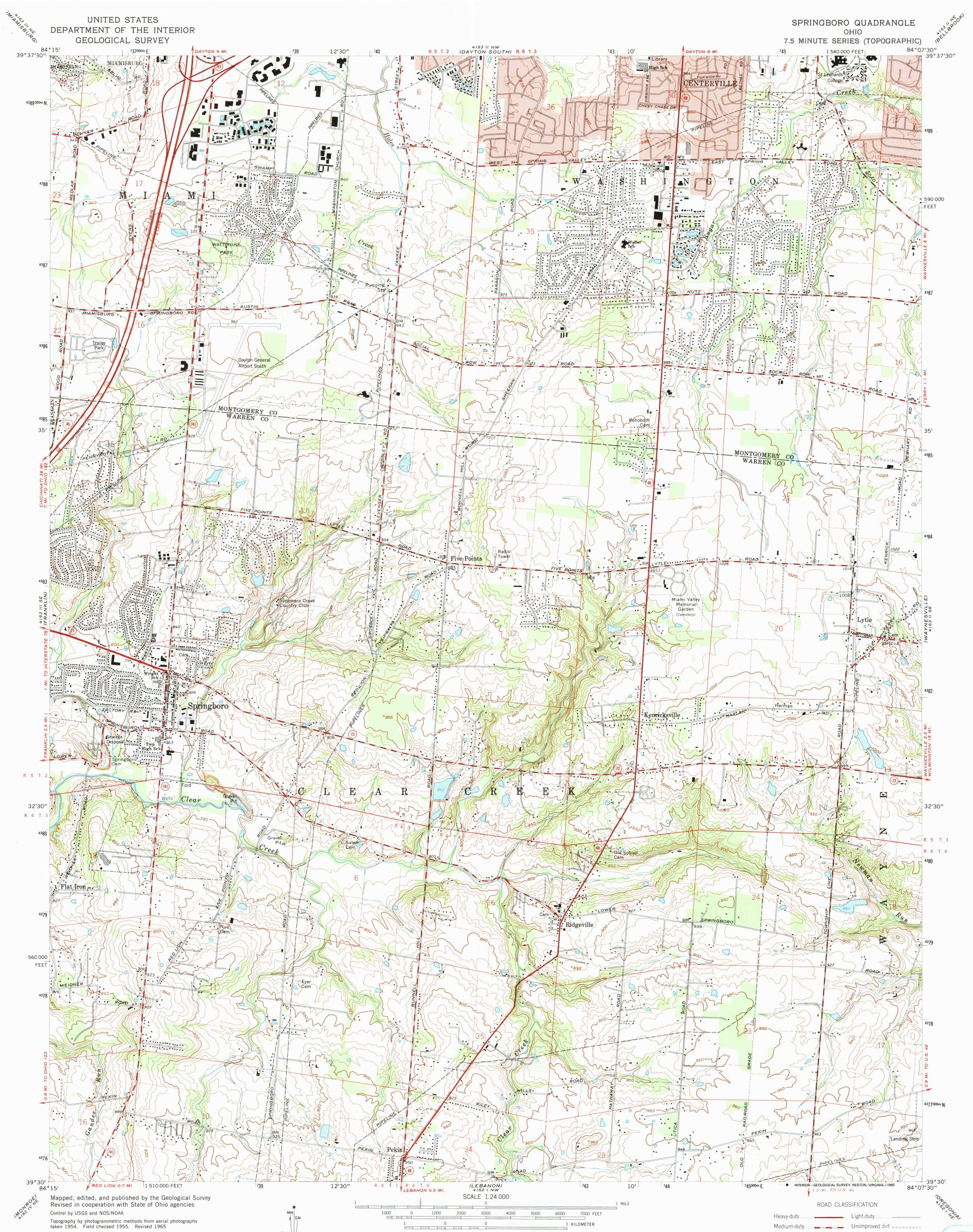
Polyconic projection. 10,000-foot grid ticks based on Ohio coordinate system, south zone. 1000-meter Universal Transverse Mercator grid ticks, zone 16, shown in blue. 1927 North American Datum.
