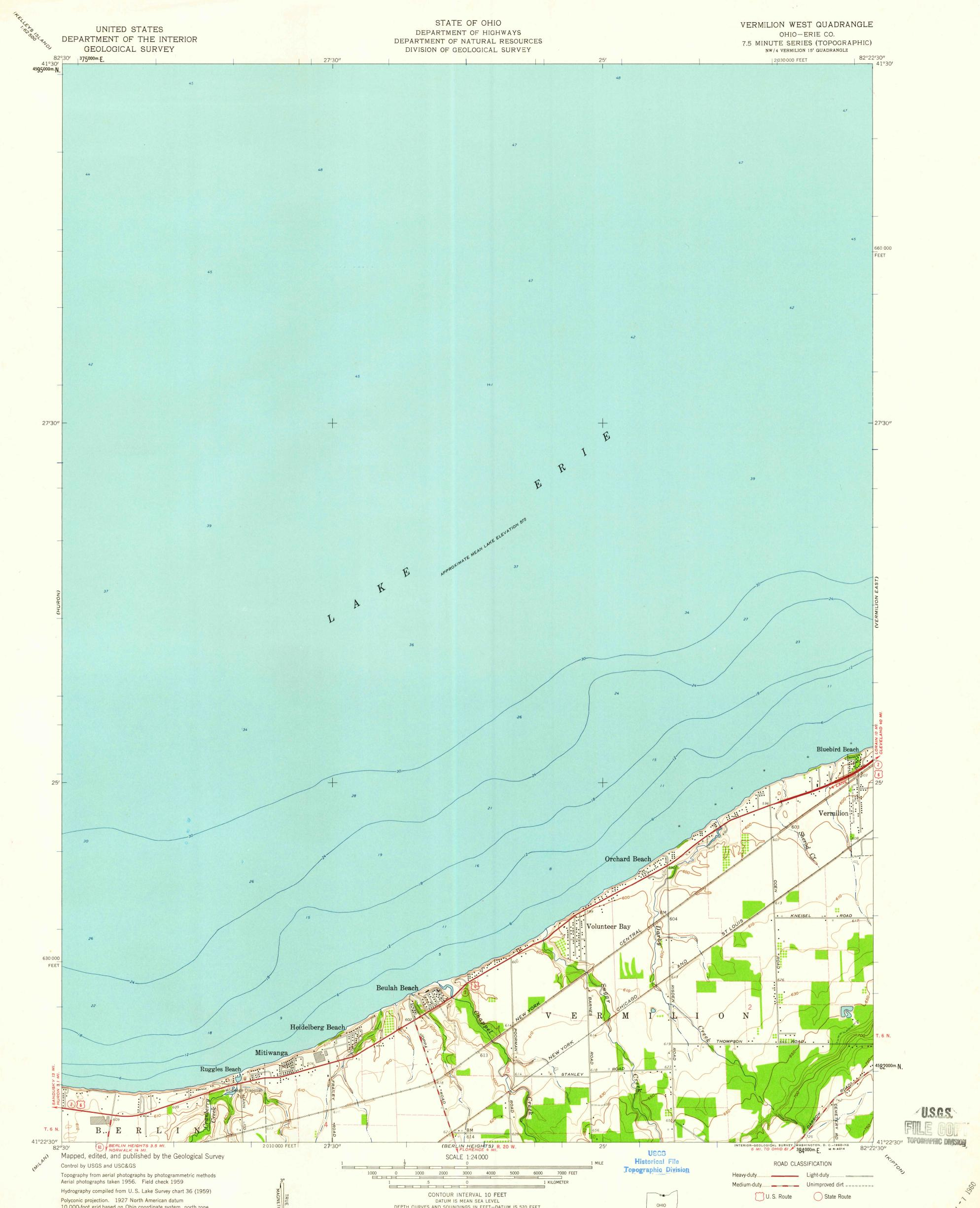
Aerial photographs taken 1956. Field check 1959 Hydrography compiled from U.S. Lake Survey chart 36 (1959) Polyconic projection. 1927 North American datum 10,000-foot grid based on Ohio coordinate system, north zone 1,000-meter Universal Transverse Mercator grid ticks, zone 17, shown in blue Dotted land lines established by private subdivision of the Connecticut Western Reserve
