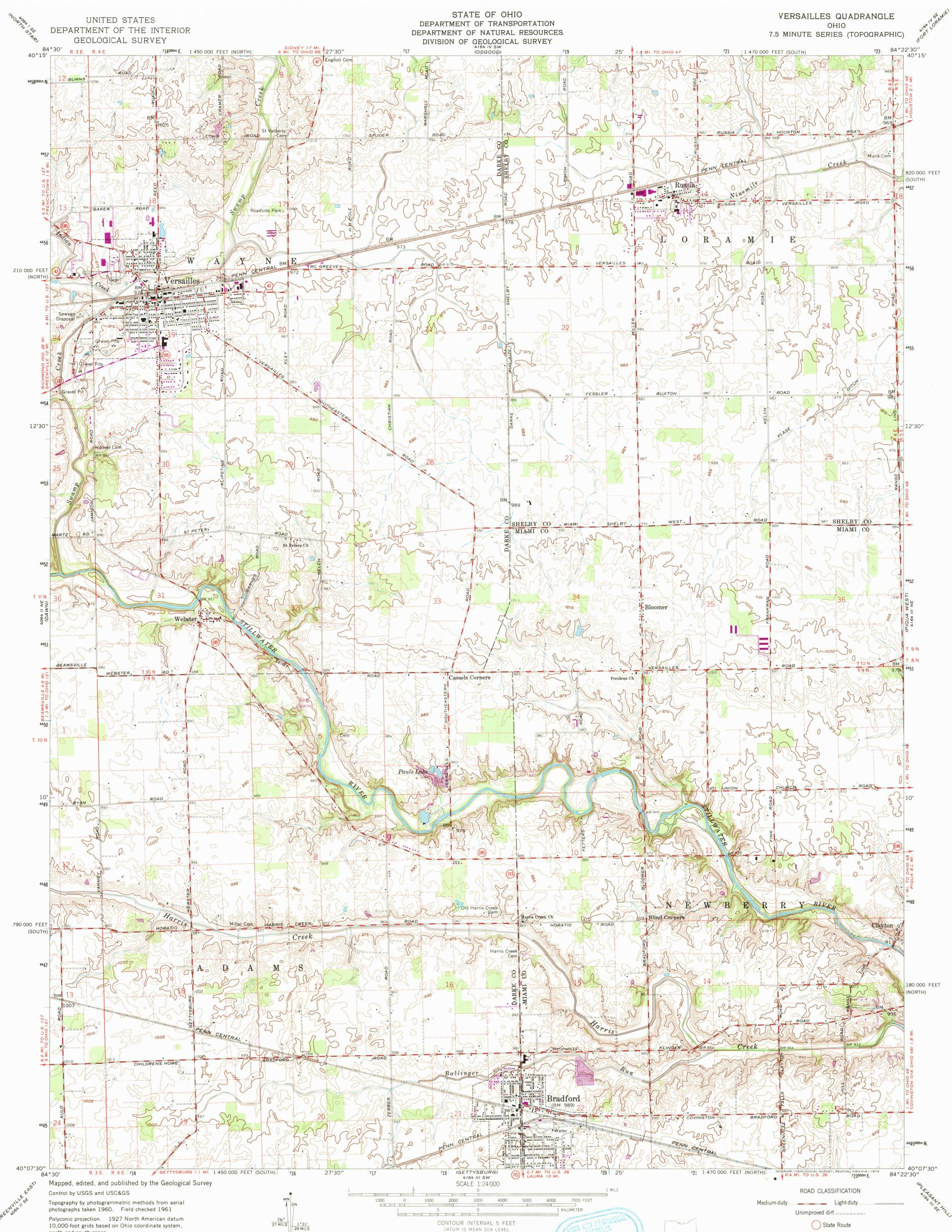
Polyconic projection. 1927 North American datum 10,000-foot grids based on Ohio coordinate system, north and south zones 1000-meter Universal Transverse Mercator grid ticks, zone 16, shown in blue
