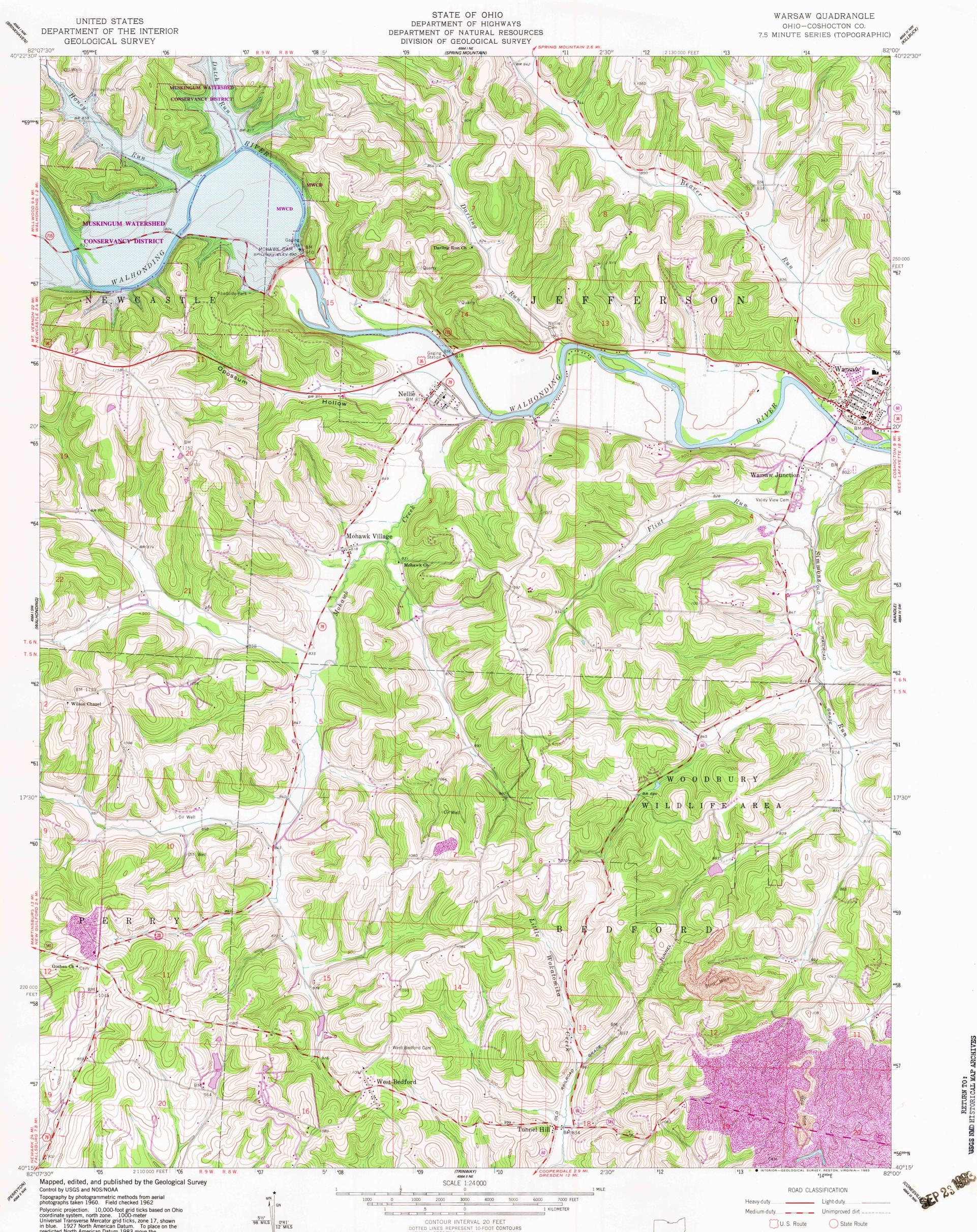
coordinate system, north zone. 1000-meter Universal Transverse Mercator grid ticks, zone 17, shown in blue. 1927 North American Datum. To place on the predicted North American Datum 1983 move the projection lines 3 meters south and 12 meters west as shown by dashed corner ticks
