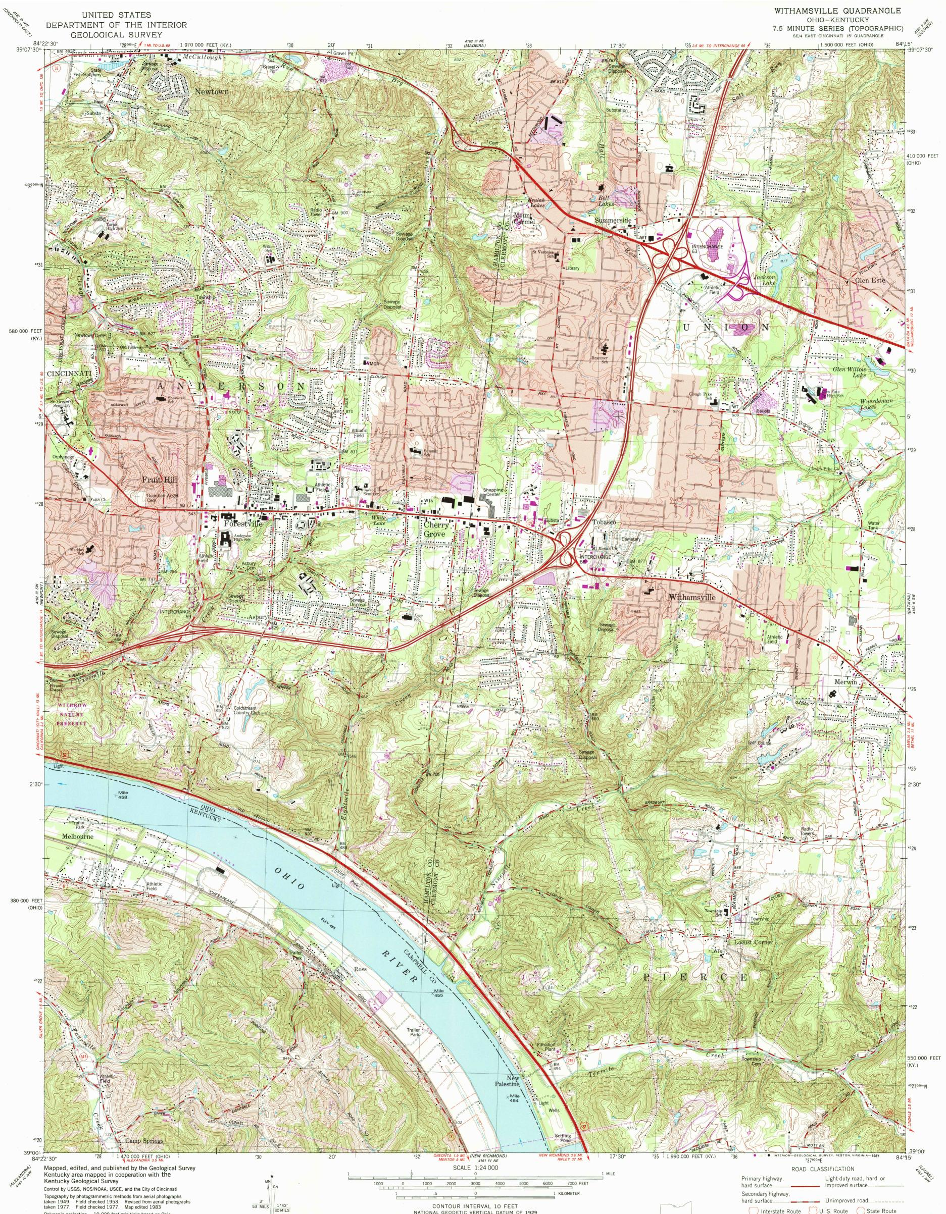
Polyconic projection. 10,000-foot grid ticks based on Ohio coordinate system, south zone and Kentucky coordinate system, north zone. 1000-meter Universal Transverse Mercator grid, To place on the predicted North American Datum move the projection lines 3 meters south and 6 meters west as shown by dashed corner ticks
