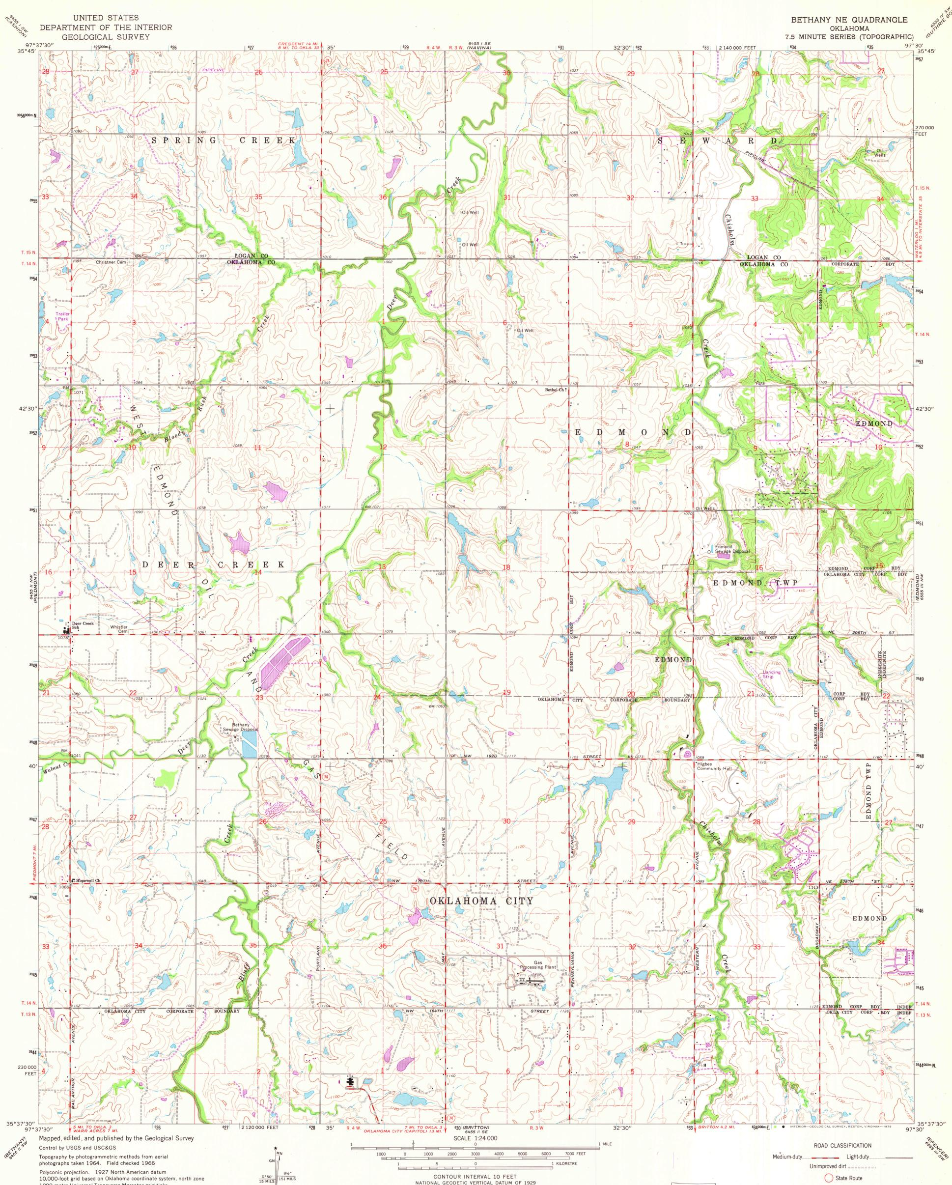
Polyconic projection. 1927 North American datum 10,000-foot grid based on Oklahoma coordinate system, north zone 1000-metre Universal Transverse Mercator grid ticks, zone 14, shown in blue
