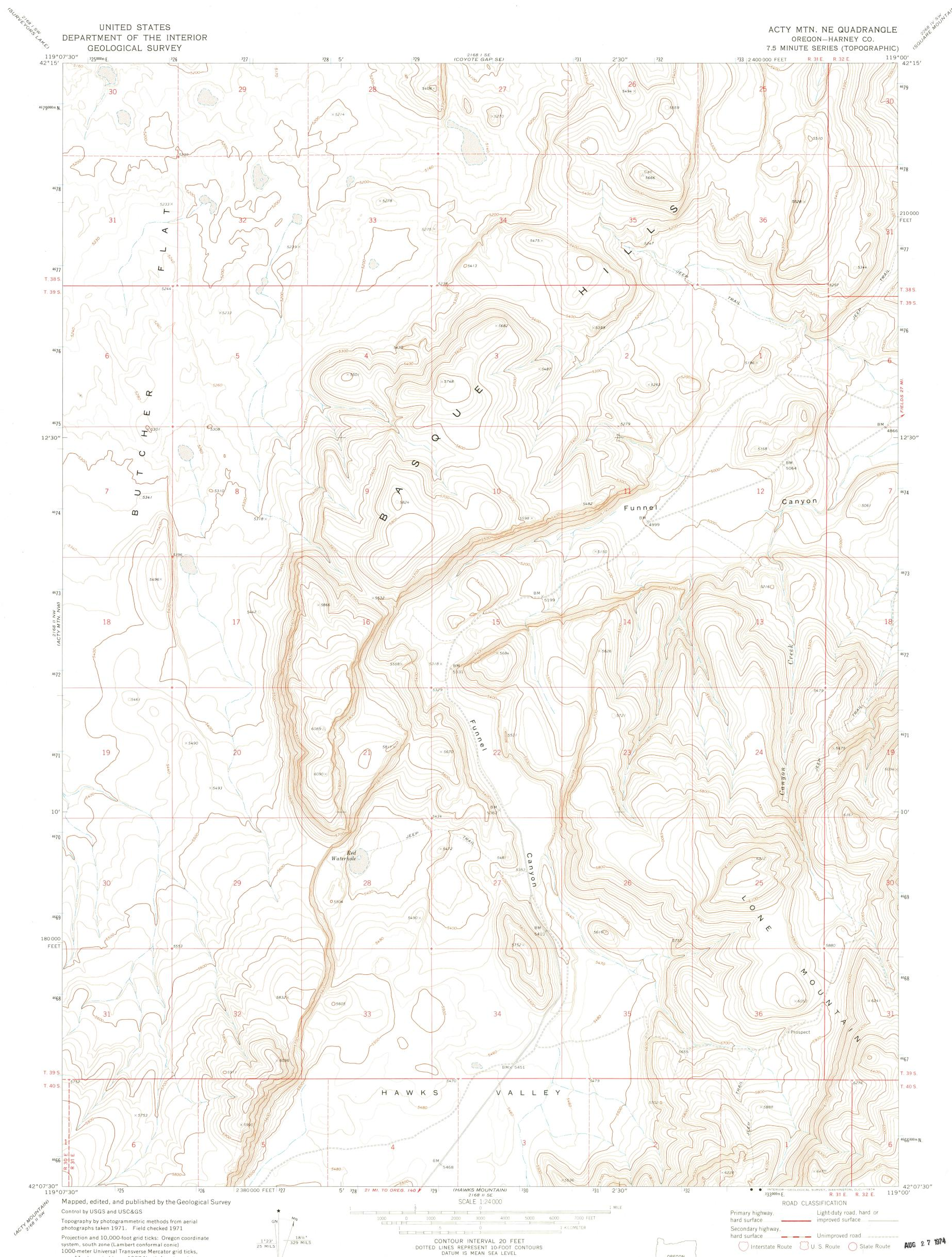
Projection and 10,000-foot grid ticks: Oregon coordinate system, south zone (Lambert conformal conic) 1000-meter Universal Transverse Mercator grid ticks, zone 11, shown in blue. 1927 North American datum Fine red dashed lines indicate selected fence lines
