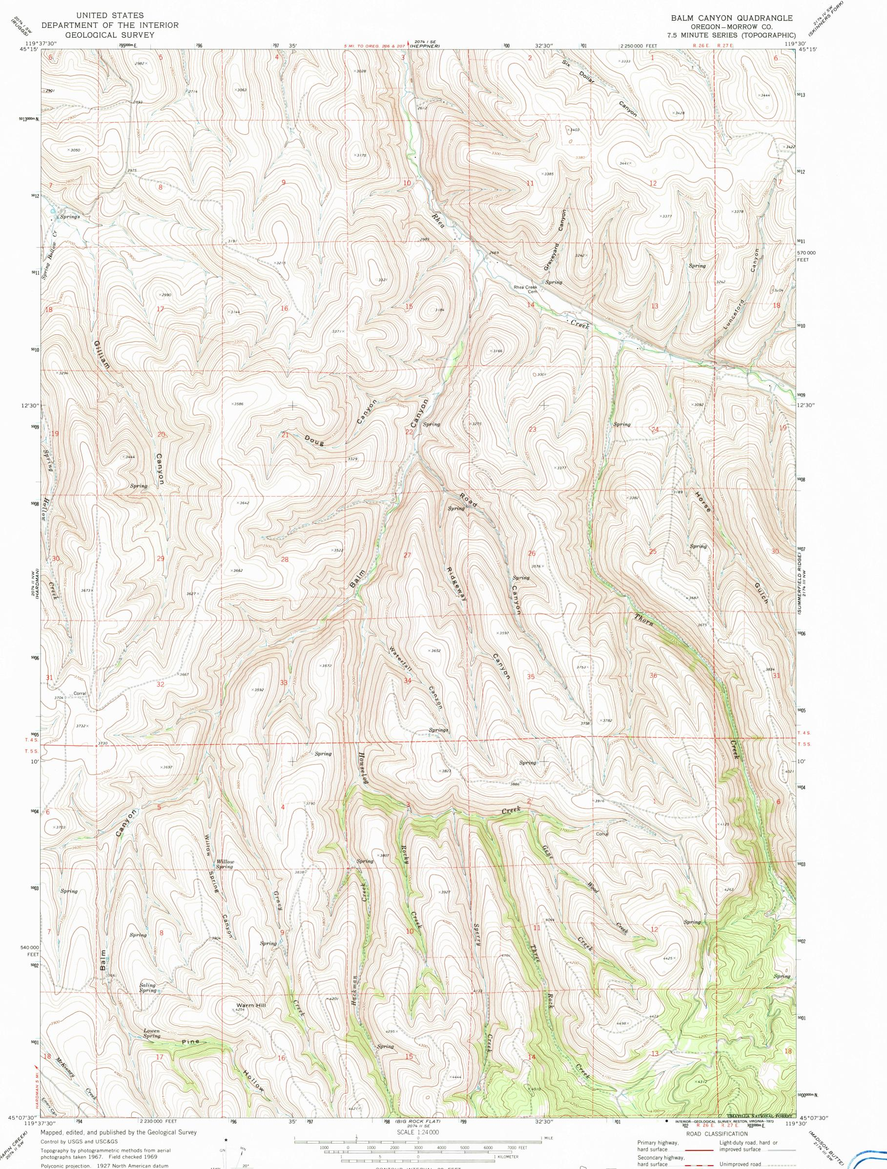
Polyconic projection. 1927 North American datum 1°49' 32 MILS 356 MILS 10,000-foot grid based on Oregon coordinate system, north zone 1000-meter Universal Transverse Mercator grid ticks, zone 11, shown in blue UTM GRID AND 1969 MAGNETIC NORTH DECLINATION AT CENTER OF SHEET Fine red dashed lines indicate selected fence lines
