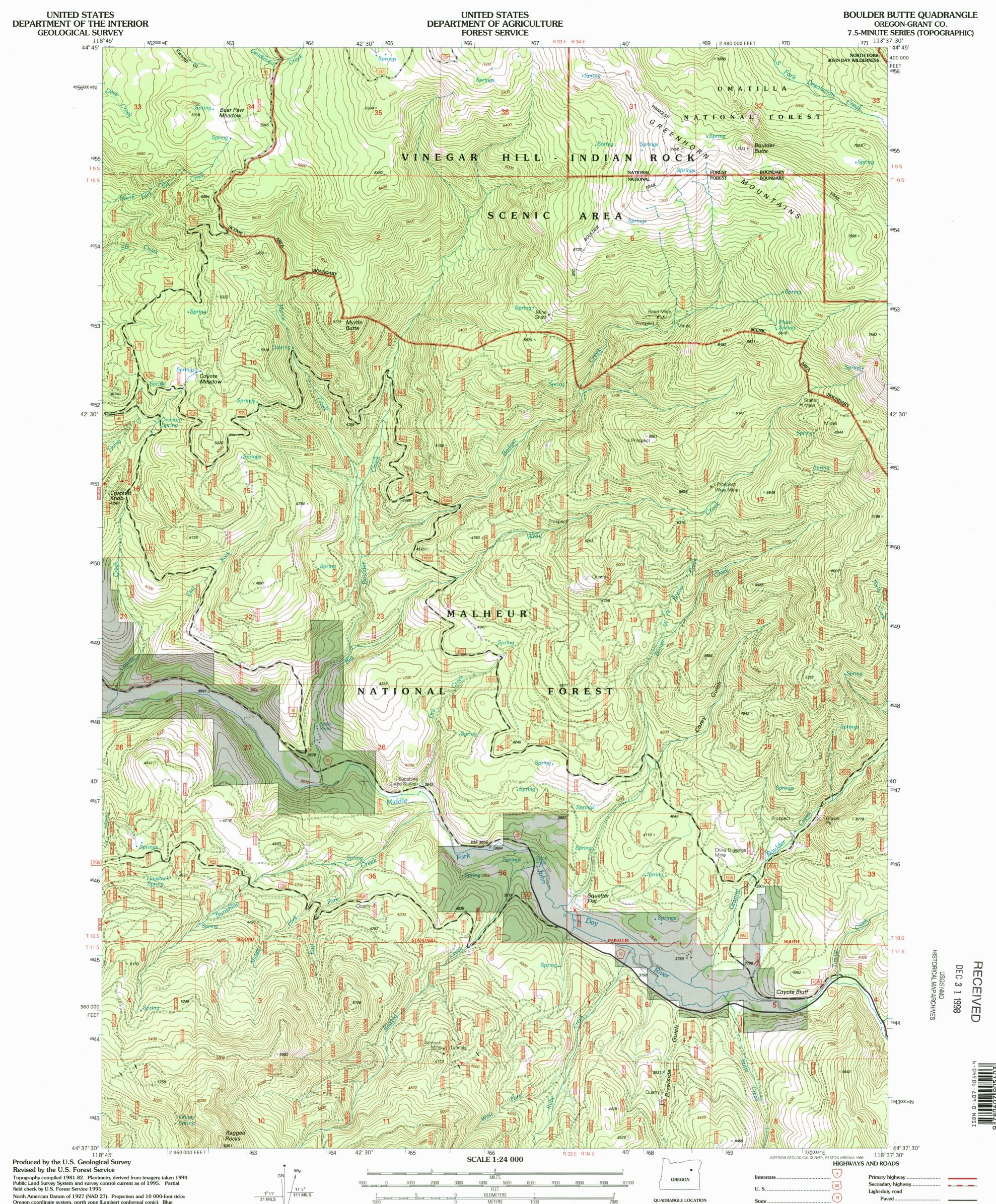
Oregon coordinate system, north zone (Lambert conformal conic). Blue 1000-meter Universal Transverse Mercator ticks, zone 11
