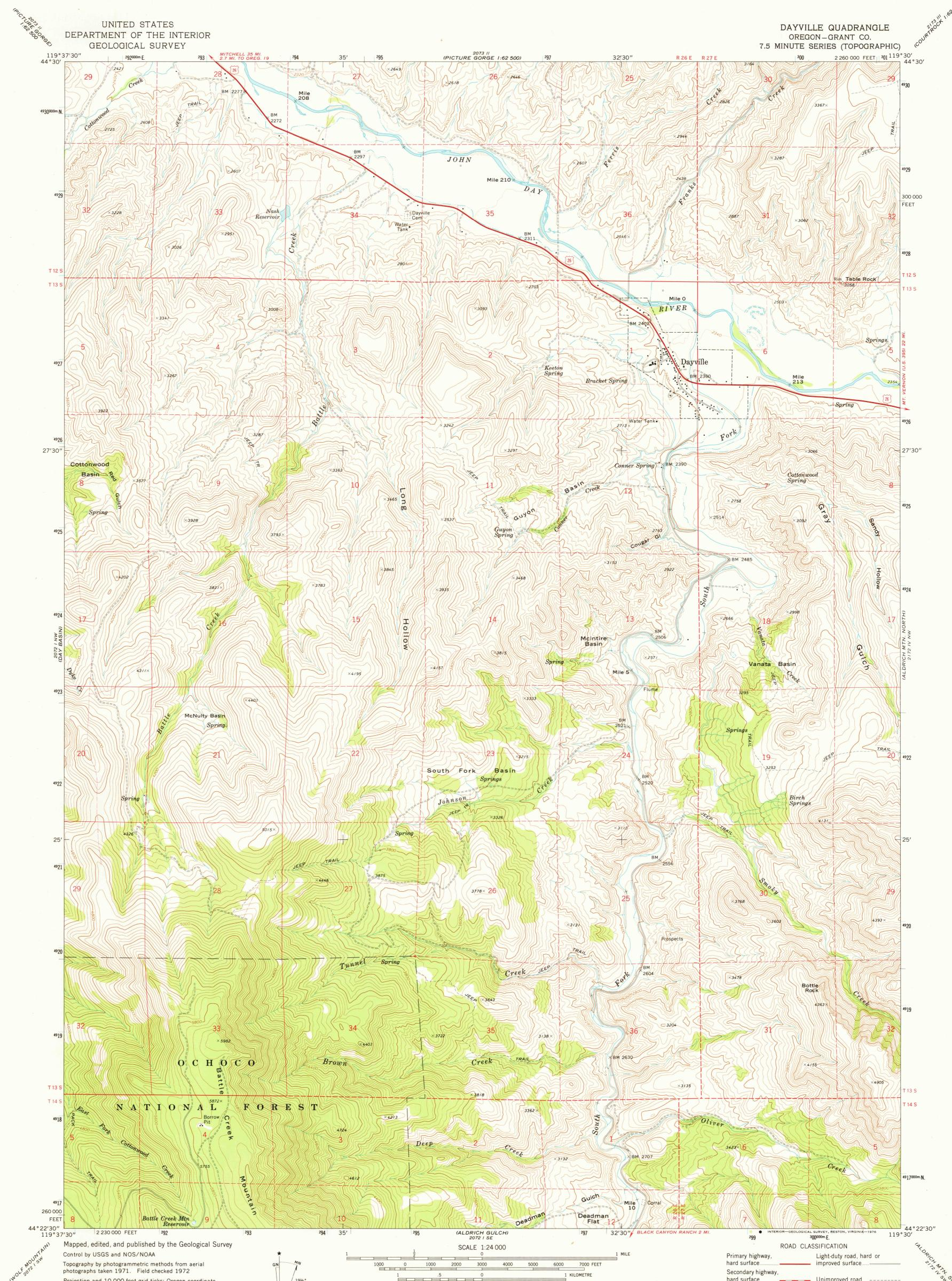
Projection and 10,000-foot grid ticks: Oregon coordinate system, north zone (Lambert conformal conic) 1000-metre Universal Transverse Mercator grid ticks, zone 11, shown in blue. 1927 North American datum
