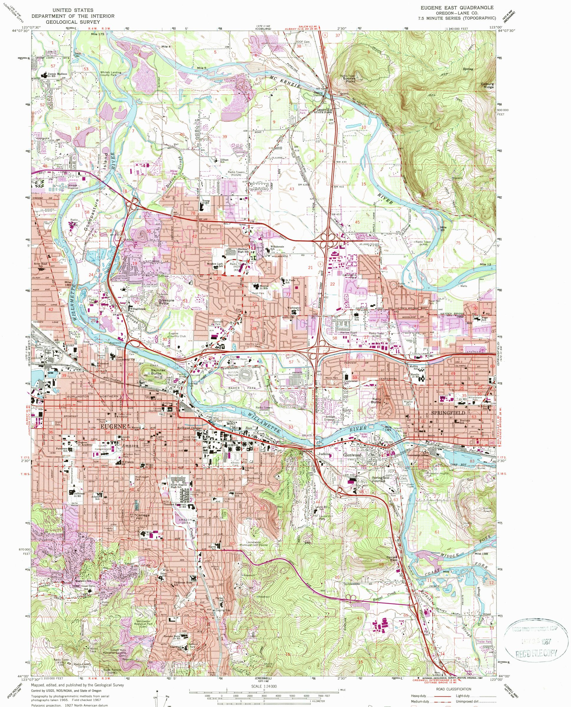
10,000-foot grid based on Oregon coordinate system, south zone 1000-meter Universal Transverse Mercator grid ticks, zone 10, shown in blue
