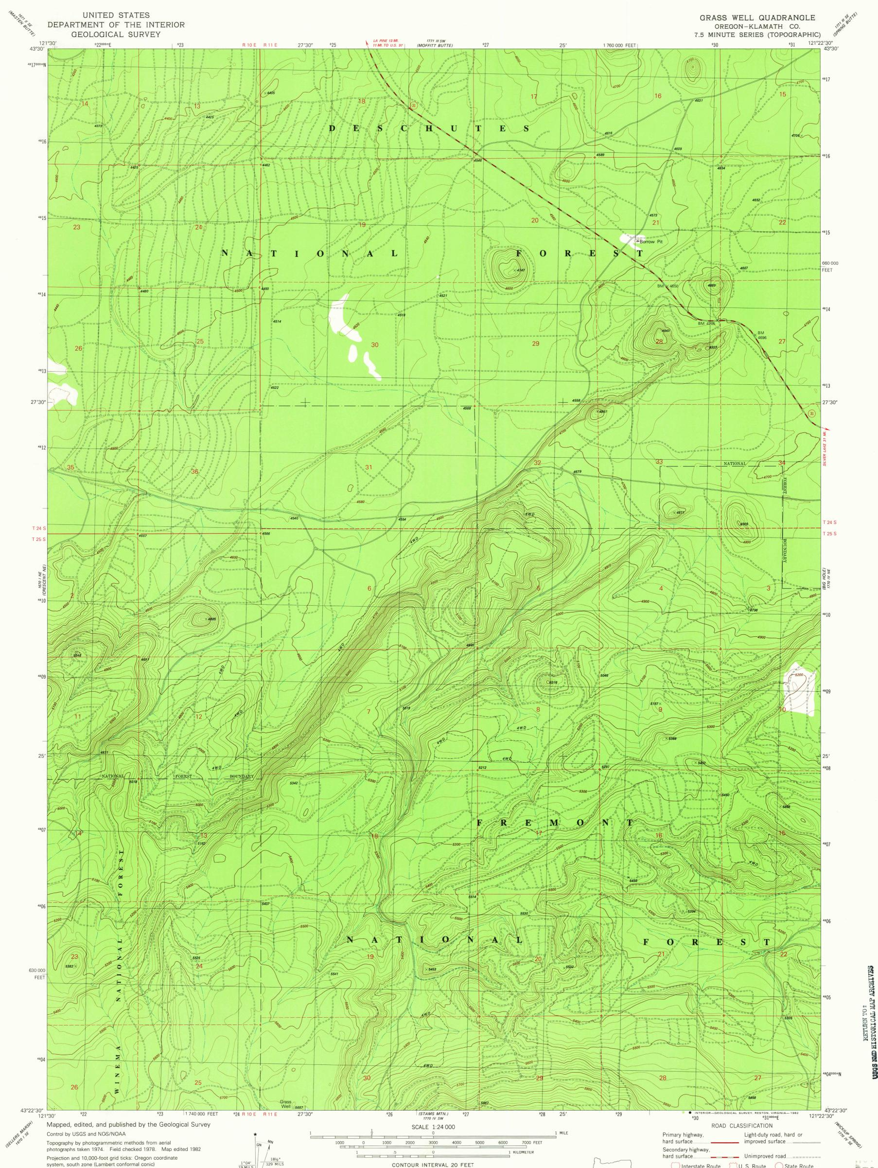
Projection and 10,000-foot grid ticks: Oregon coordinate system, south zone (Lambert conformal conic) 1000-meter Universal Transverse Mercator grid, zone 10 1927 North American Datum To place on the predicted North American Datum 1983 move the projection lines 20 meters north and 92 meters east as shown by dashed corner ticks There may be private inholdings within the boundaries of
