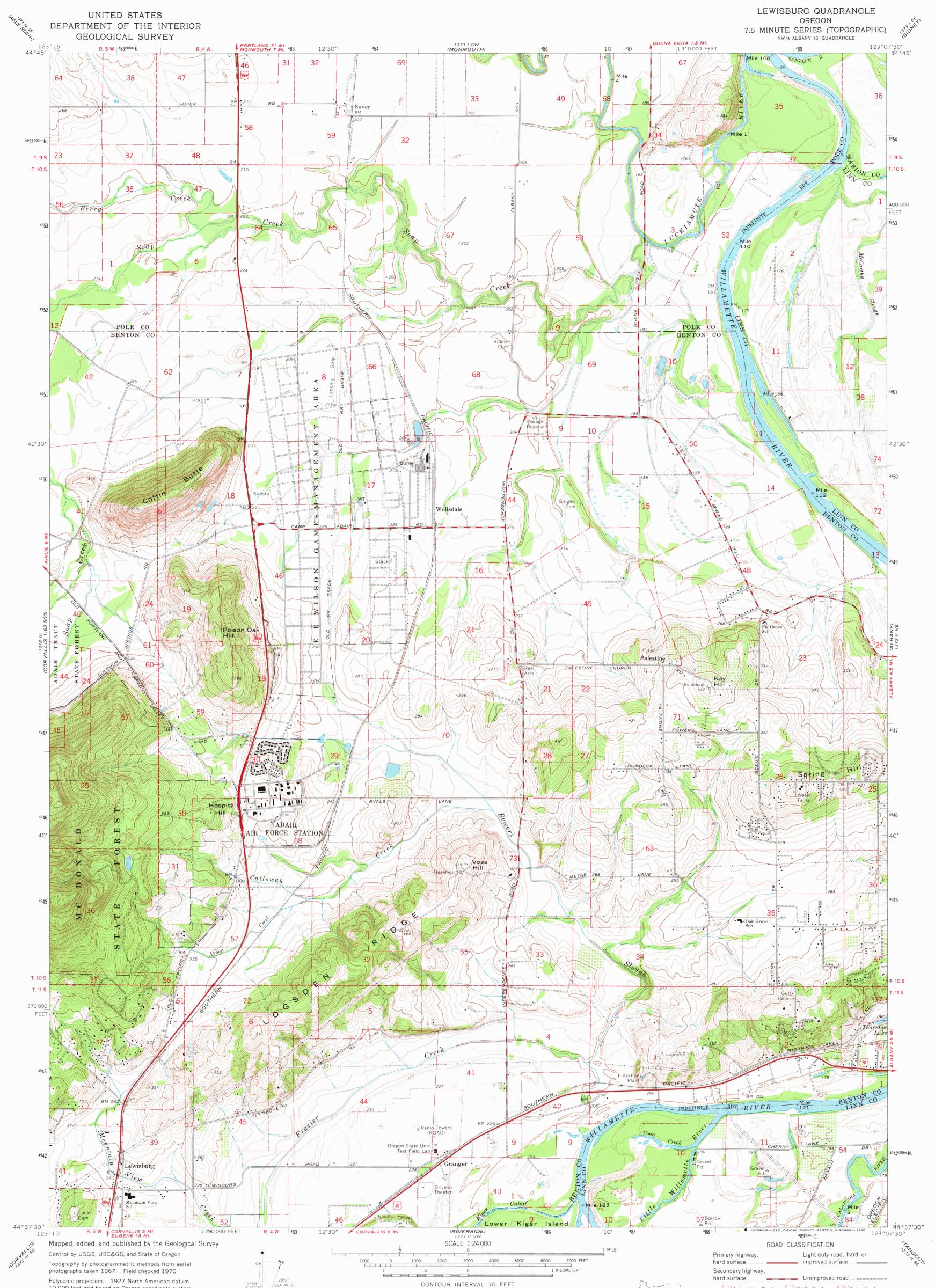
10,000-foot grid based on Oregon coordinate system, north zone 1000-meter Universal Transverse Mercator grid ticks, zone 10, shown in blue UTM GRID AND 1970 MAGNETIC NORTH DECLINATION AT CENTER OF SHEET To place on the predicted North American Datum 1983 move the projection lines 23 meters north and 95 meters east as shown by dashed corner ticks There may be private inholdings within the boundaries of the National or State reservations shown on this map
