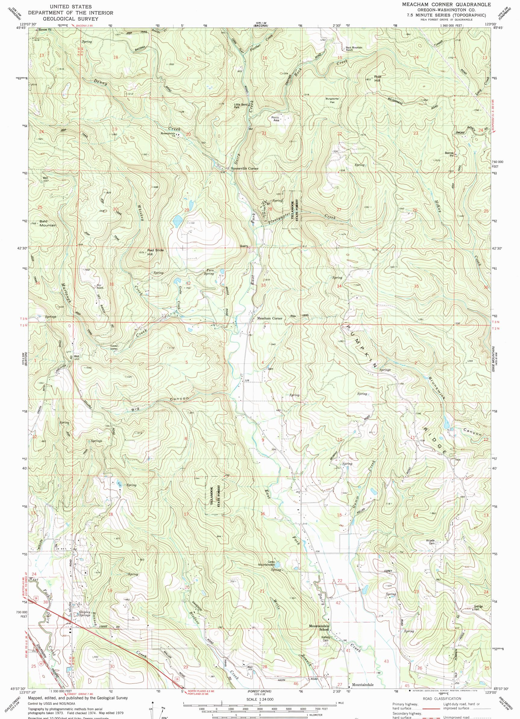
Projection and 10,000-foot grid ticks: Oregon coordinate system, north zone (Lambert conformal conic) 1000-meter Universal Transverse Mercator grid, zone 10 1927 North American datum To place on the predicted North American Datum 1983 move the projection lines 23 meters north and 95 meters east as shown by dashed corner ticks
