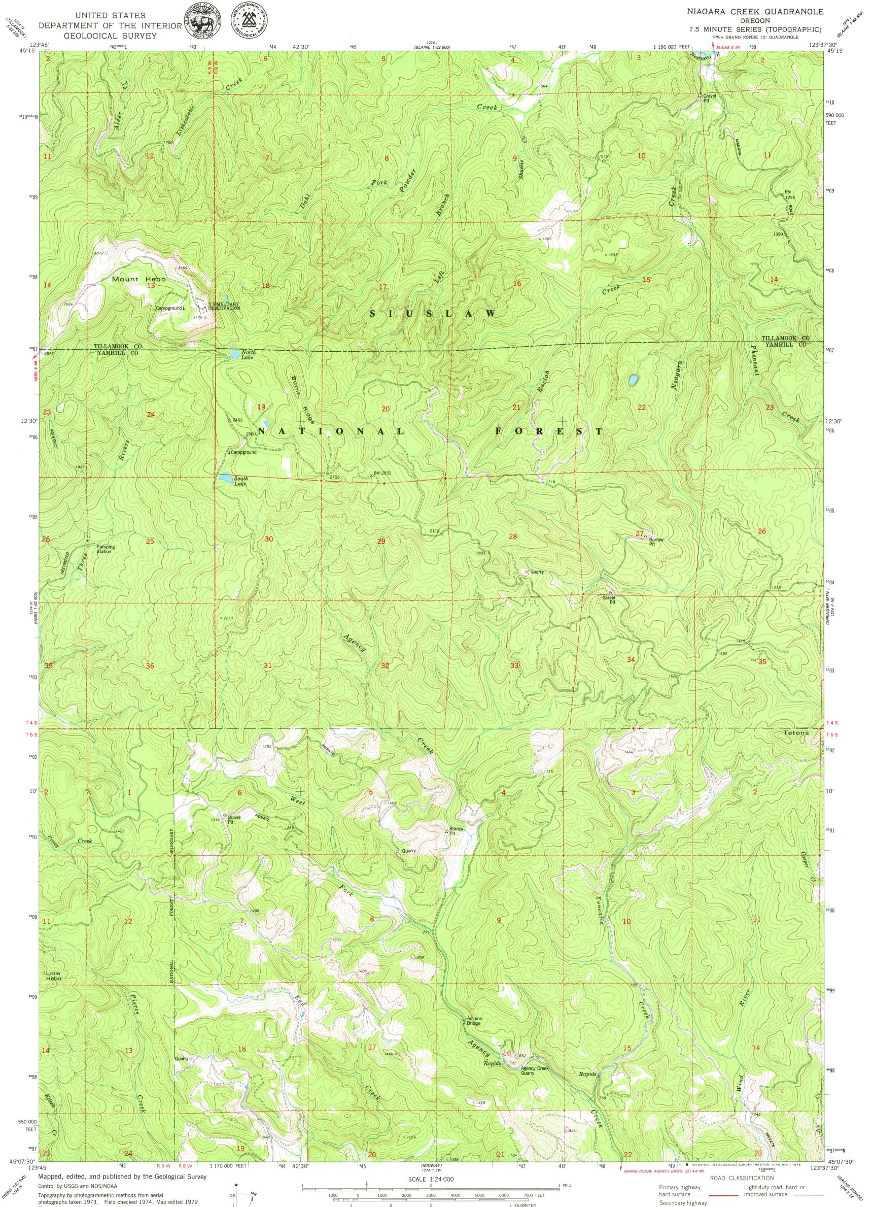
Projection and 10,000-foot grid ticks: Oregon coordinate system, north zone (Lambert conformal conic) 1000-meter Universal Transverse Mercator grid ticks, zone 10, shown in blue. 1927 North American datum To place on the predicted North American Datum 1983 move the projection lines 23 meters north and 96 meters east as shown by dashed corner ticks
