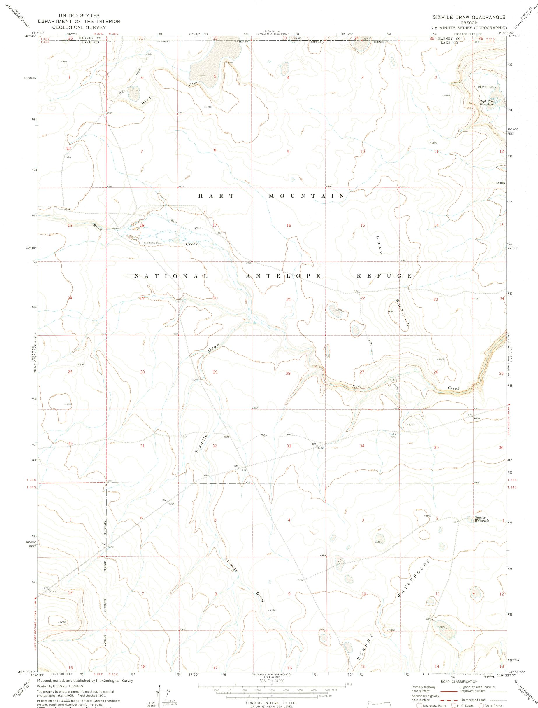
$\label{eq:projection} \mbox{ Projection and 10,000-foot grid ticks: Oregon coordinate}$ system, south zone (Lambert conformal conic) 1000-meter Universal Transverse Mercator grid ticks, zone 11, shown in blue. 1927 North American datum
