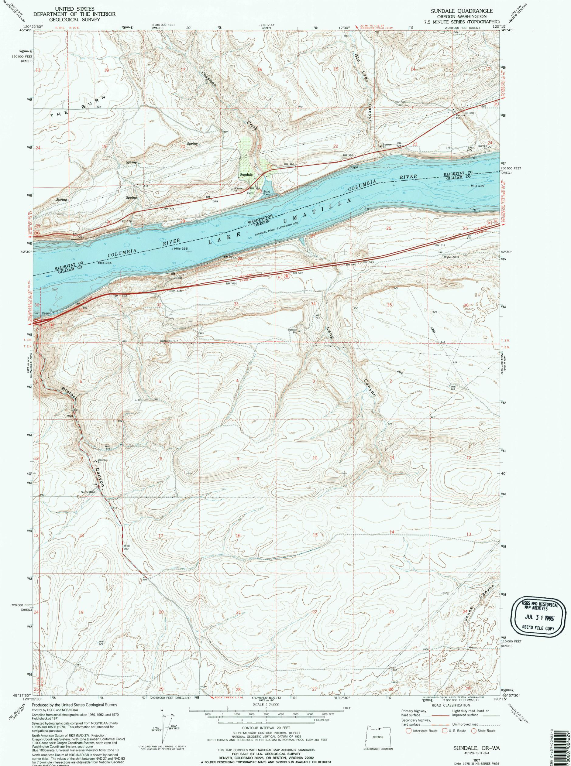
North American Datum of 1983 (NAD 83) is shown by dashed corner ticks. The values of the shift between NAD 27 and NAD 83 for 7.5-minute intersections are obtainable from National Geodetic Survey NADCON software
