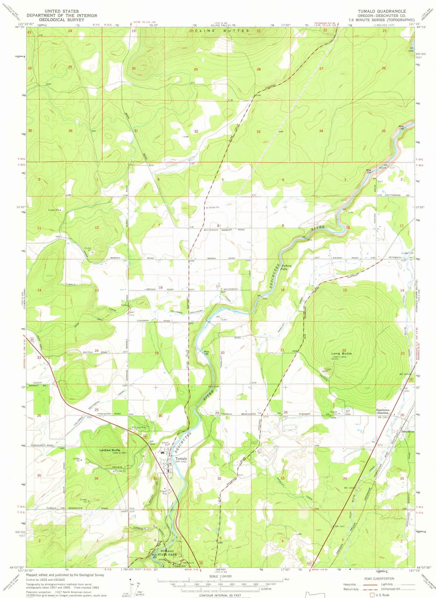
10,000-foot grid based on Oregon coordinate system, south zone 1000-metre Universal Transverse Mercator grid ticks, zone 10, shown in blue
