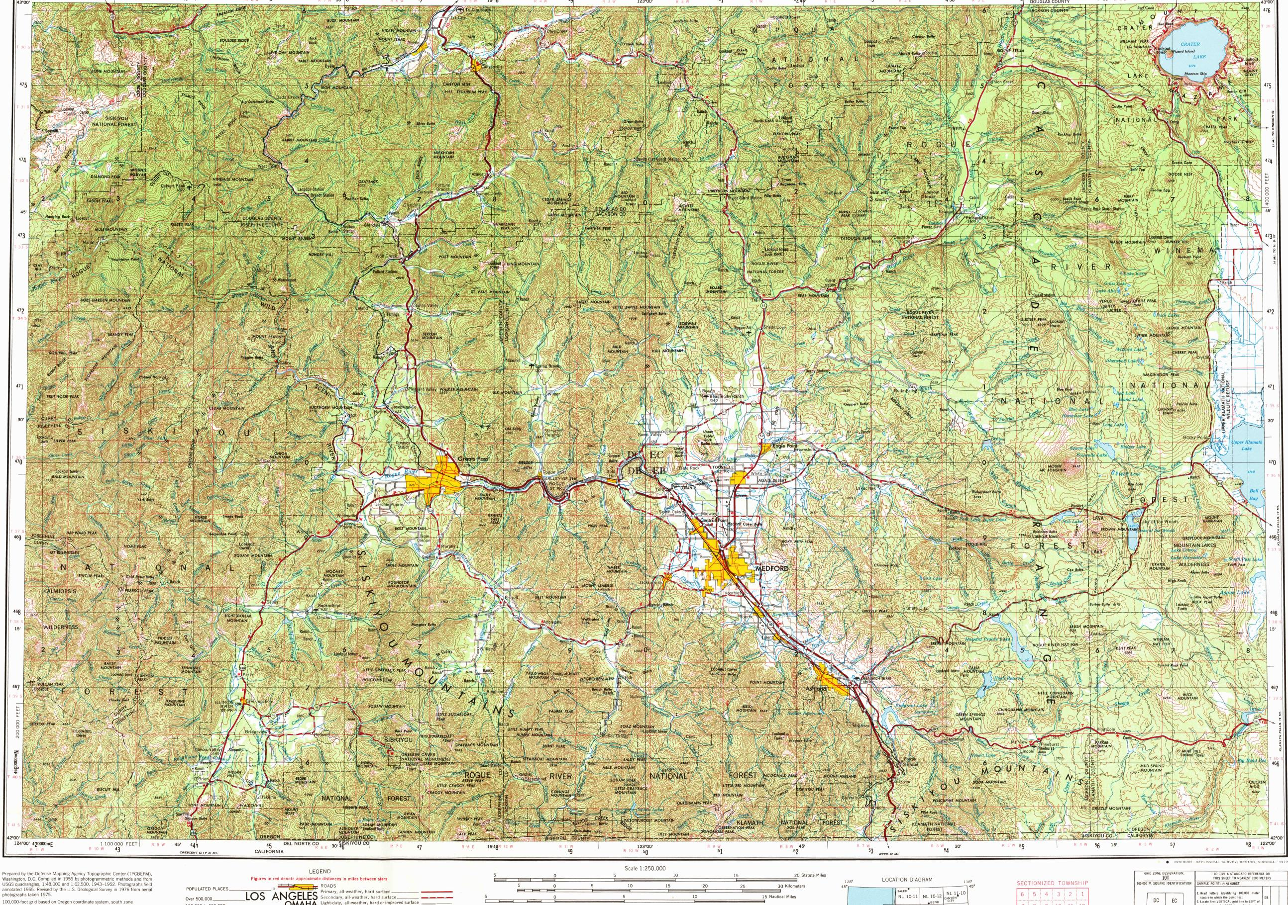
Prepared by the Defense Mapping Agency Topographic Center (TPCBEPM), Washington, D.C. Compiled in 1956 by photogrammetric methods and from USGS quadrangles, 1:48,000 and 1:62,500, 1943–1952. Photographs field annotated 1955. Revised by the U.S. Geological Survey in 1976 from aerial photographs taken 1975.
