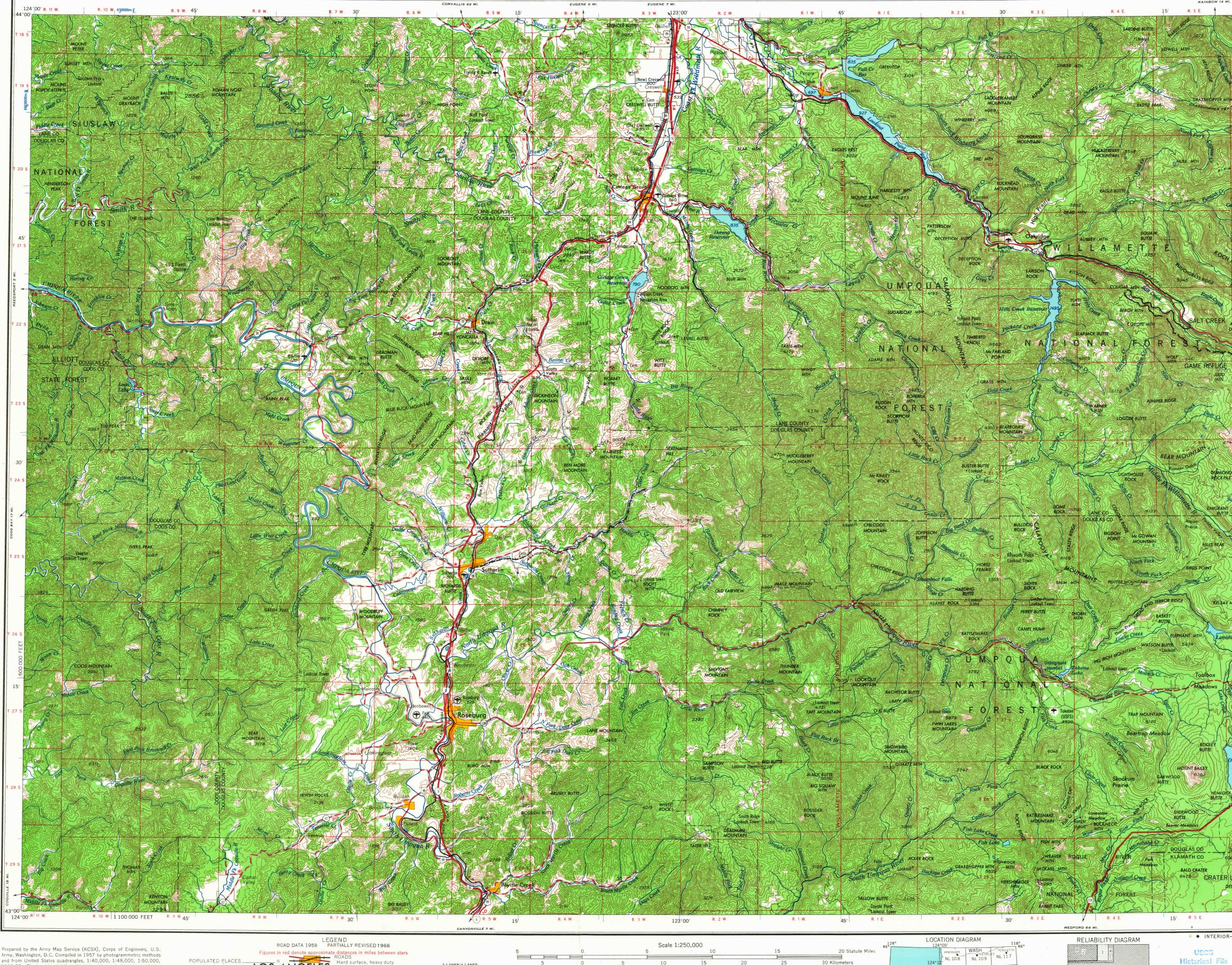
Prepared by the Army Map Service (KCSX), Corps of Engineers, U.S. Army, Washington, D.C. Compiled in 1957 by photogrammetric methods and from United States quadrangles, 1:40,000, 1:48,000, 1:50,000, 1938-55. Planimetric detail revised by photo-planimetric methods. Horizontal and vertical control by USGS, USC&GS, and Oregon State Highway Department. Map field checked 1958. Limited revision by U.S. Geological Survey1966. 100,000-foot grid based on Oregon coordinate system, south zone
