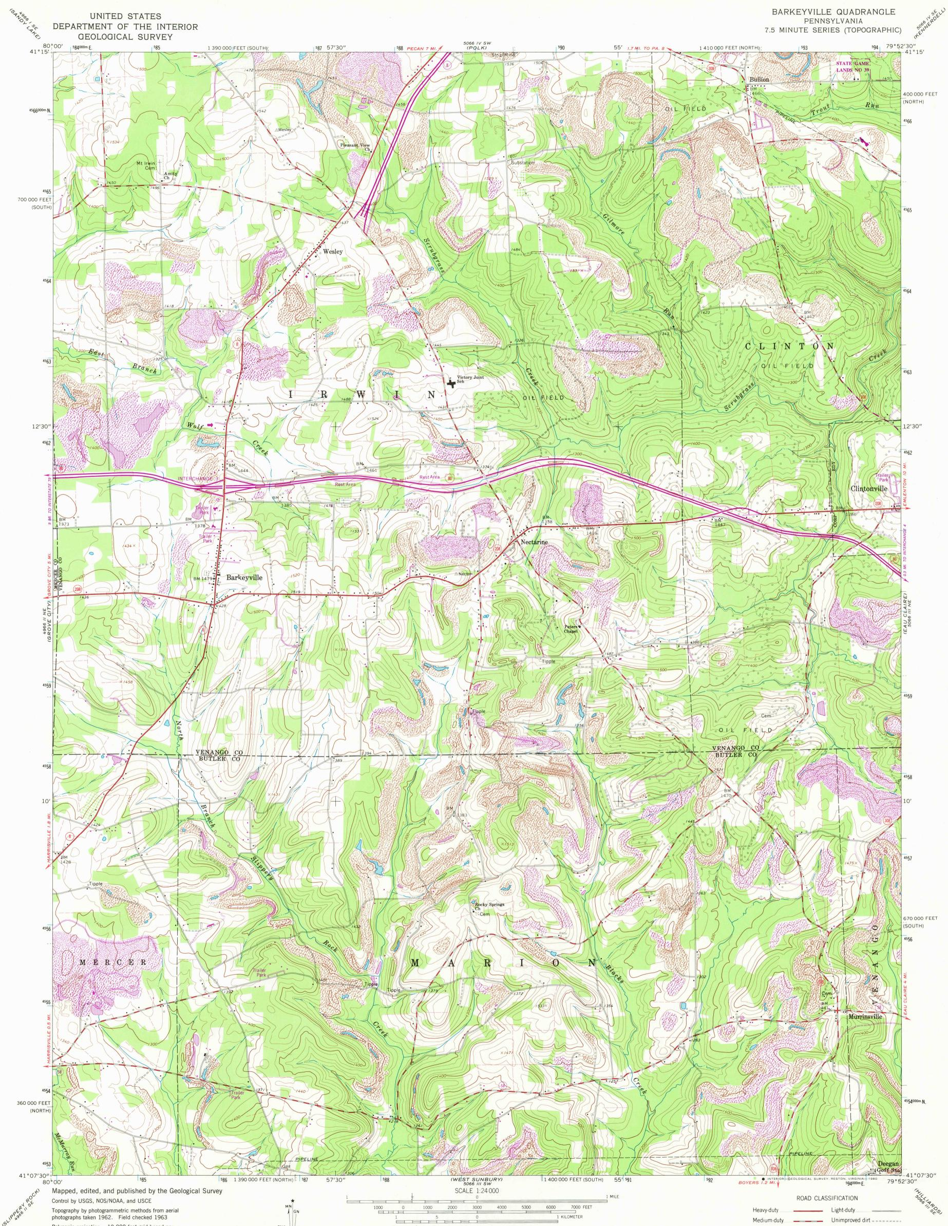
Polyconic projection. 10,000-foot grid based on Pennsylvania coordinate system, north and south zones 1000-meter Universal Transverse Mercator grid ticks, zone 17, shown in blue. 1927 North American Datum To place on the predicted North American Datum 1983 move the projection lines 3 meters south and 18 meters west as shown by dashed corner ticks
