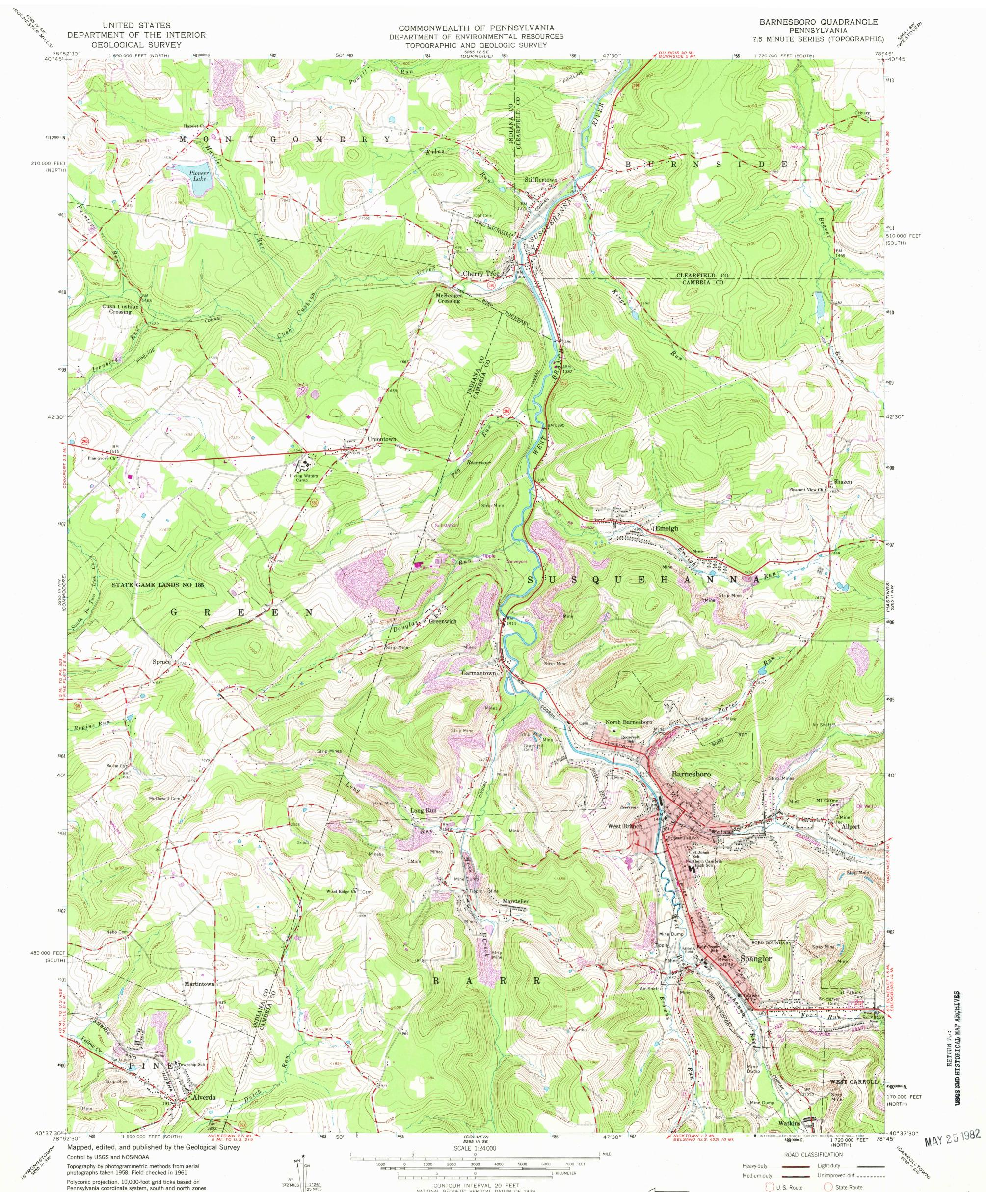
Polyconic projection. 10,000-foot grid ticks based on Pennsylvania coordinate system, south and north zones 1000-meter Universal Transverse Mercator grid ticks, zone 17, shown in blue. 1927 North American Datum To place on the predicted North American Datum 1983 move the projection lines 4 meters south and 21 meters west as shown by dashed corner ticks
