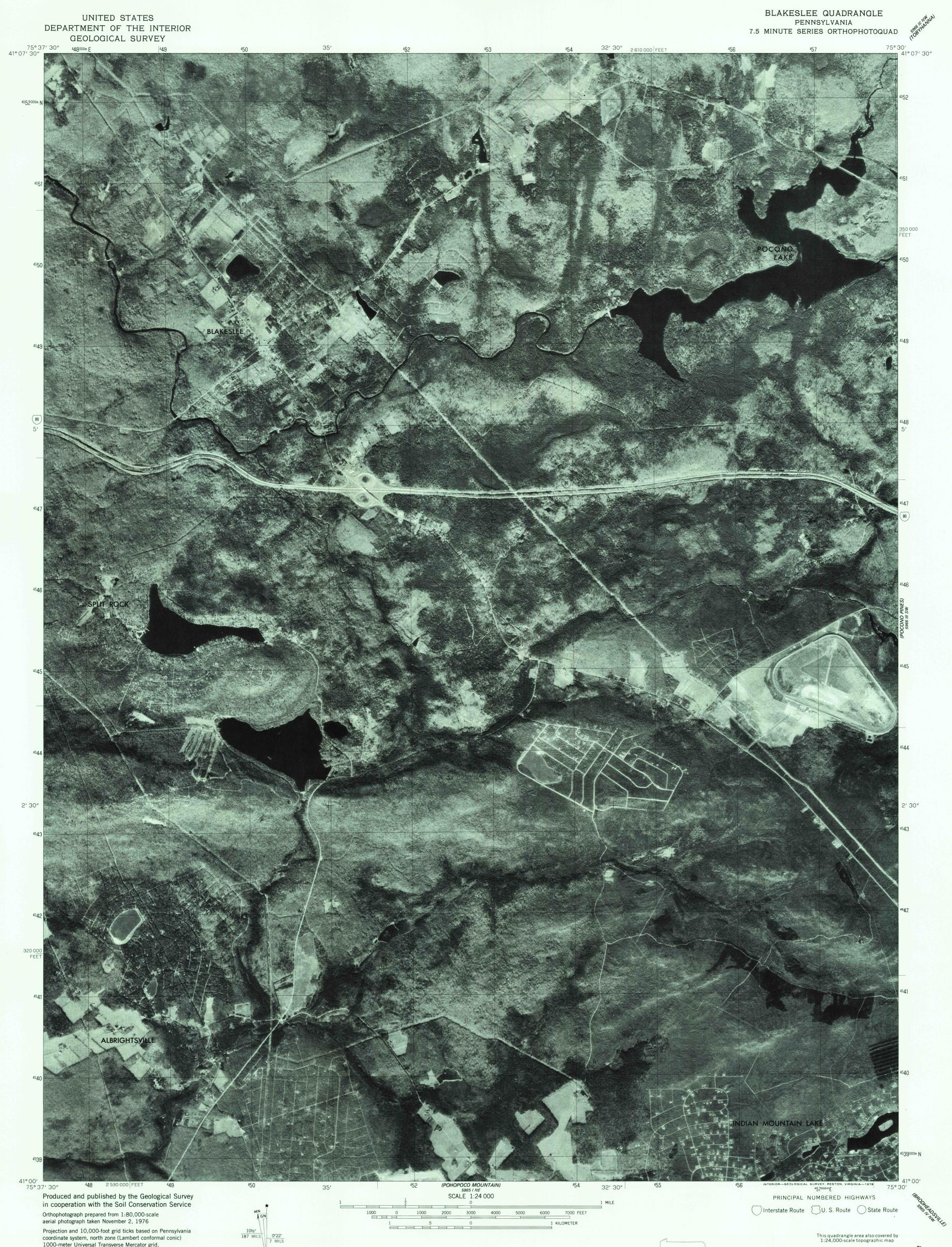
Projection and 10,000-foot grid ticks based on Pennsylvania coordinate system, north zone (Lambert conformal conic) 1000-meter Universal Transverse Mercator grid, zone 18. 1927 North American datum
