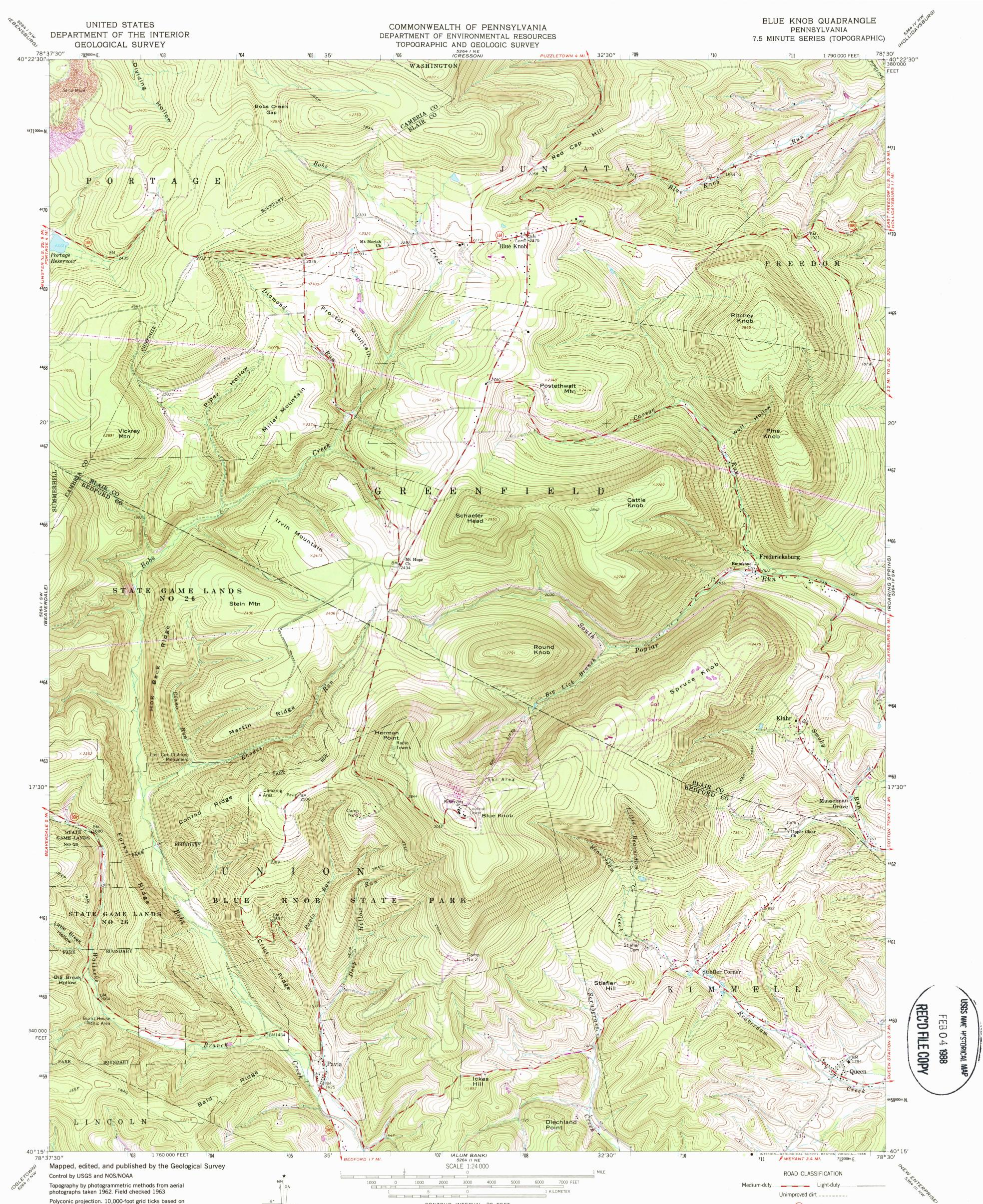
Polyconic projection. 10,000-foot grid ticks based on Pennsylvania coordinate system, south zone 1000-meter Universal Transverse Mercator grid ticks, zone 17, shown in blue. 1927 North American Datum To place on the predicted North American Datum 1983 move the projection lines 5 meters south and 22 meters west as shown by dashed corner ticks 8° 142 MILS 28 MILS
