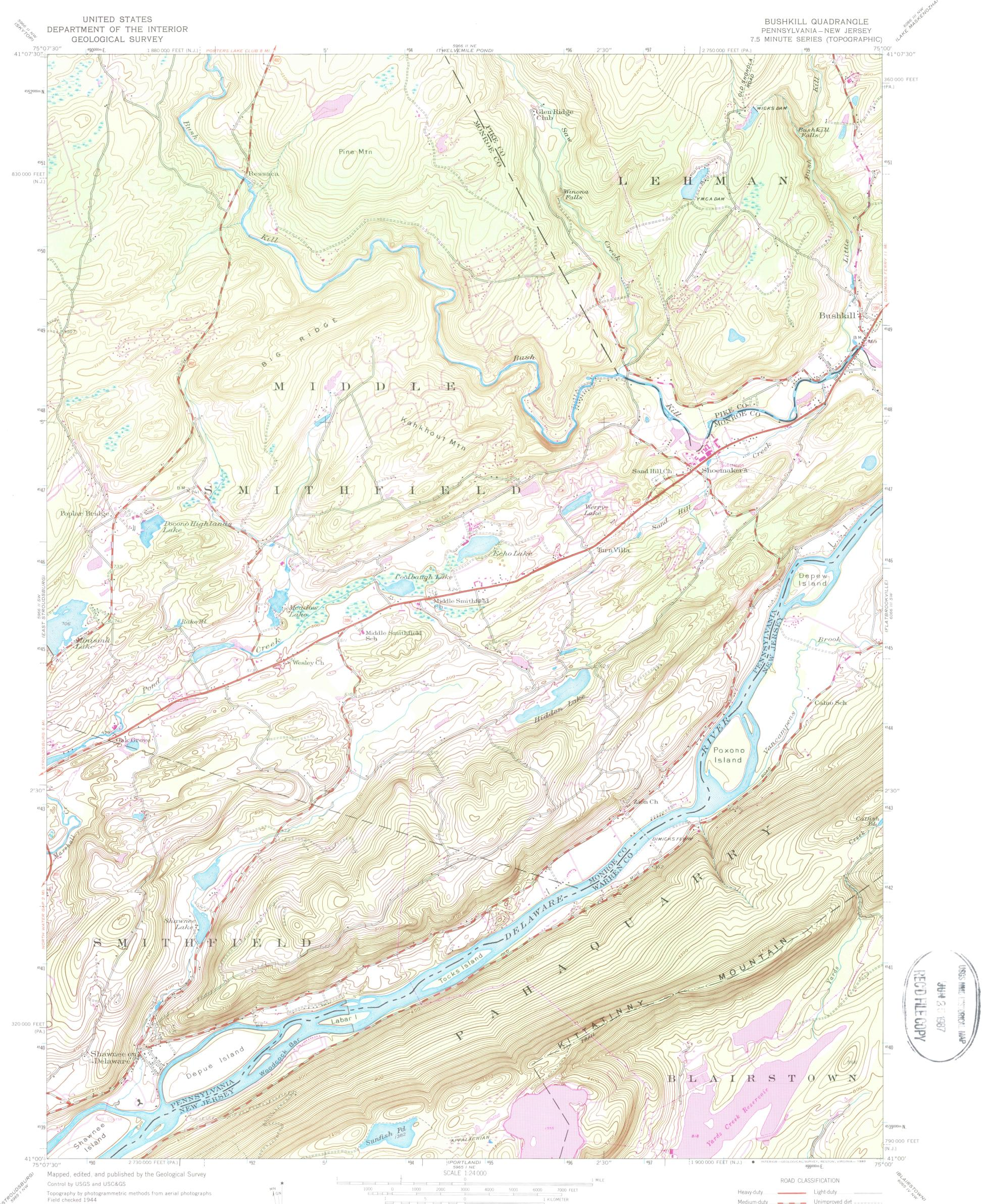
Polyconic projection. 1927 North American Datum 10,000-foot grids based on Pennsylvania coordinate system, north zone, and New Jersey coordinate system 1000-meter Universal Transverse Mercator grid ticks, zone 18, shown in blue UTM GRID AND 1973 MAGNETIC NORTH DECLINATION AT CENTER OF SHEET
