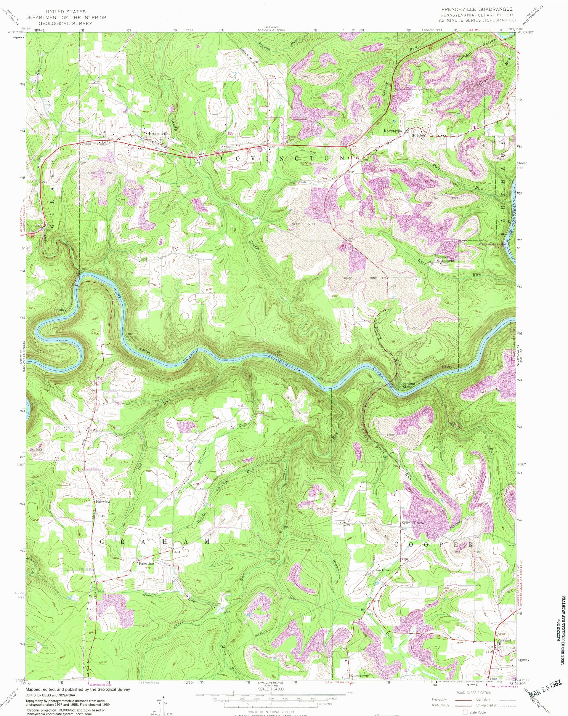
Polyconic projection. 10,000-foot grid ticks based on Pennsylvania coordinate system, north zone 1000-meter Universal Transverse Mercator grid ticks, zone 17, shown in blue. 1927 North American Datum To place on the predicted North American Datum 1983 move the projection lines 4 meters south and 23 meters west as shown by dashed corner ticks
