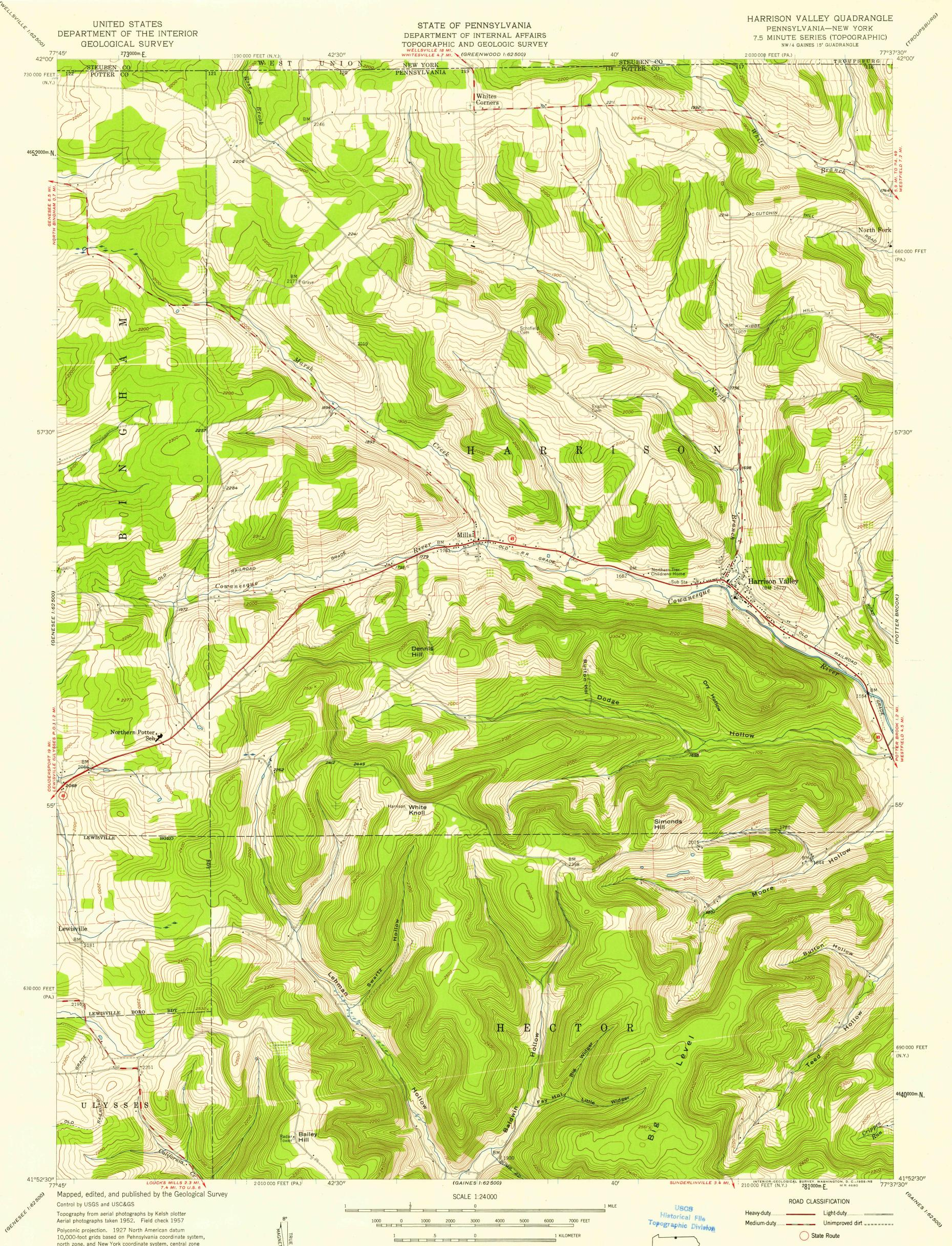
Polyconic projection. 1927 North American datum 10,000-foot grids based on Pennsylvania coordinate system, north zone, and New York coordinate system, central zone 1000-meter Universal Transverse Mercator grid ticks, zone 18, shown in blue
