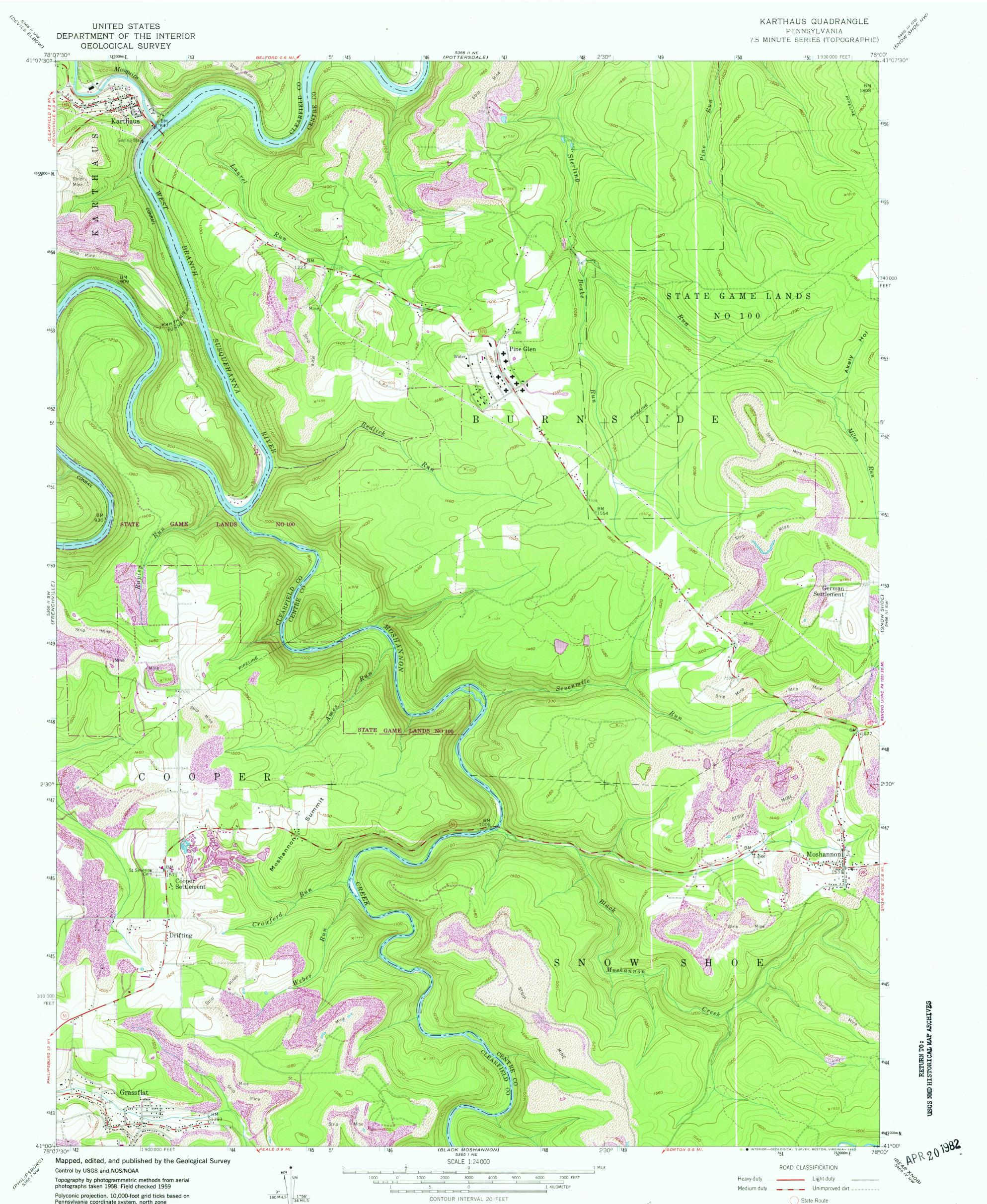
Polyconic projection. 10,000-foot grid ticks based on Pennsylvania coordinate system, north zone 1000-meter Universal Transverse Mercator grid ticks, zone 17, shown in blue. 1927 North American Datum To place on the predicted North American Datum 1983 move the projection lines 4 meters south and 23 meters west as shown by dashed corner ticks
