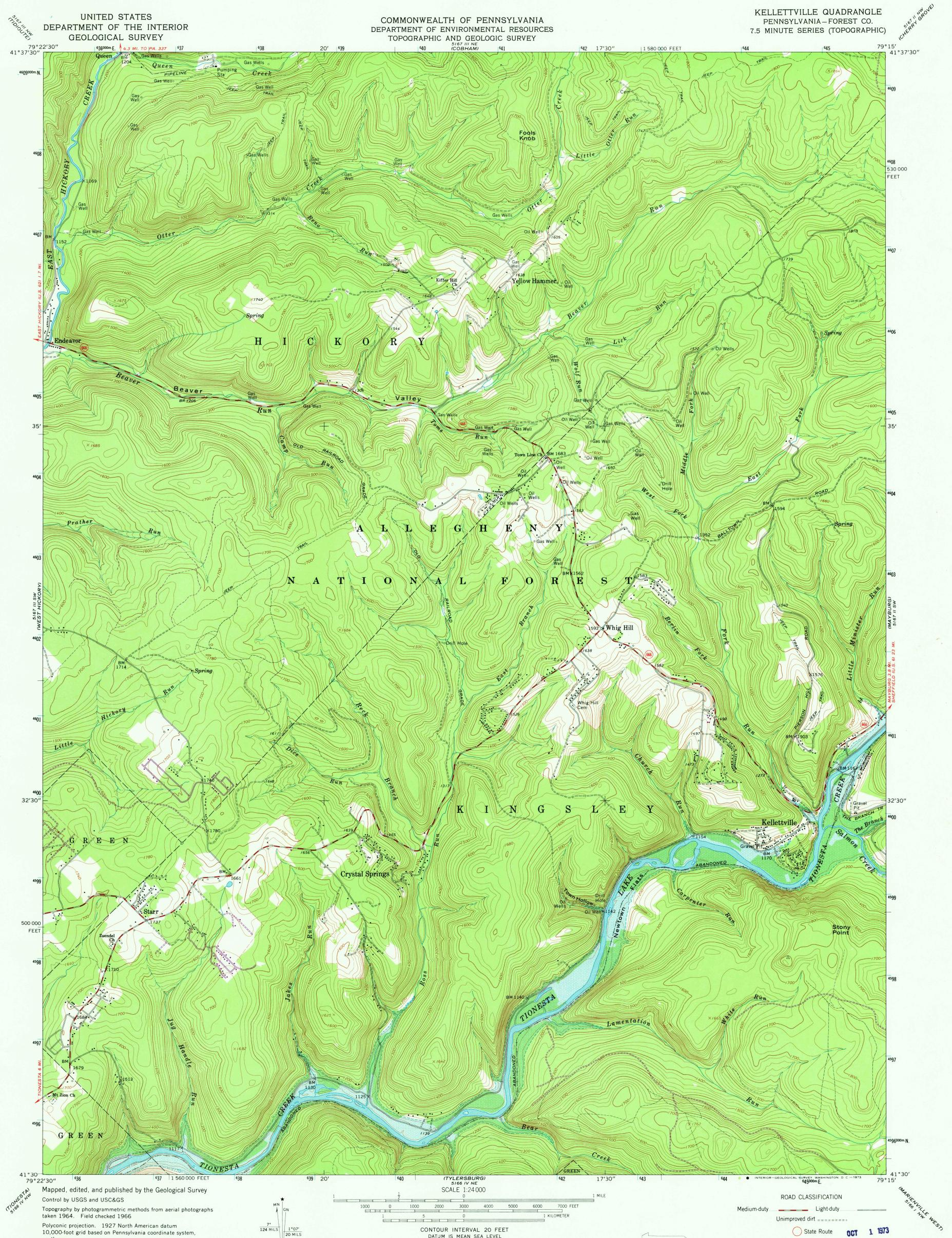
10,000-foot grid based on Pennsylvania coordinate system, north zone 1000-meter Universal Transverse Mercator grid ticks, zone 17, shown in blue
