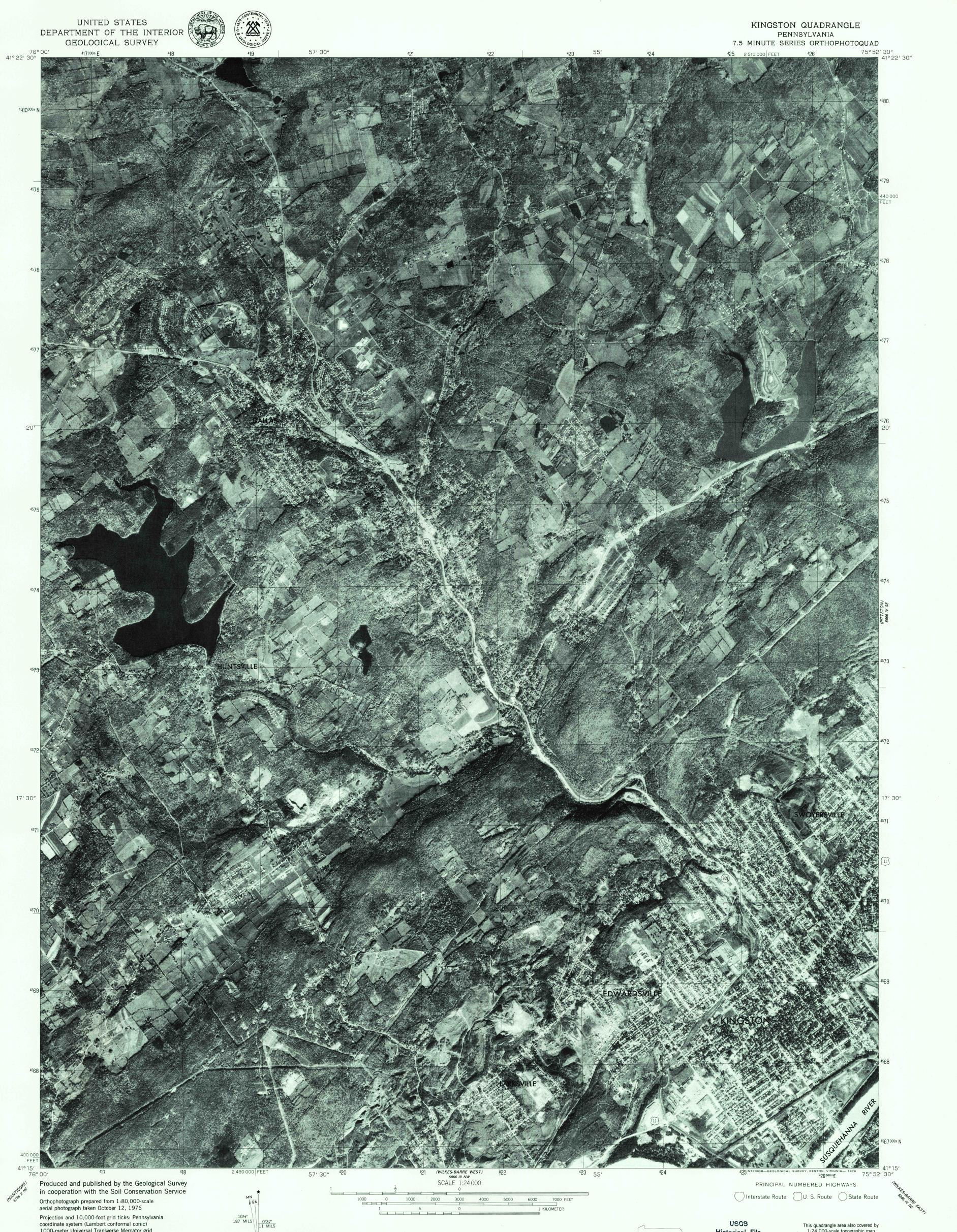
Projection and 10,000-foot grid ticks: Pennsylvania coordinate system (Lambert conformal conic) 1000-meter Universal Transverse Mercator grid zone 18. 1927 North American datum
