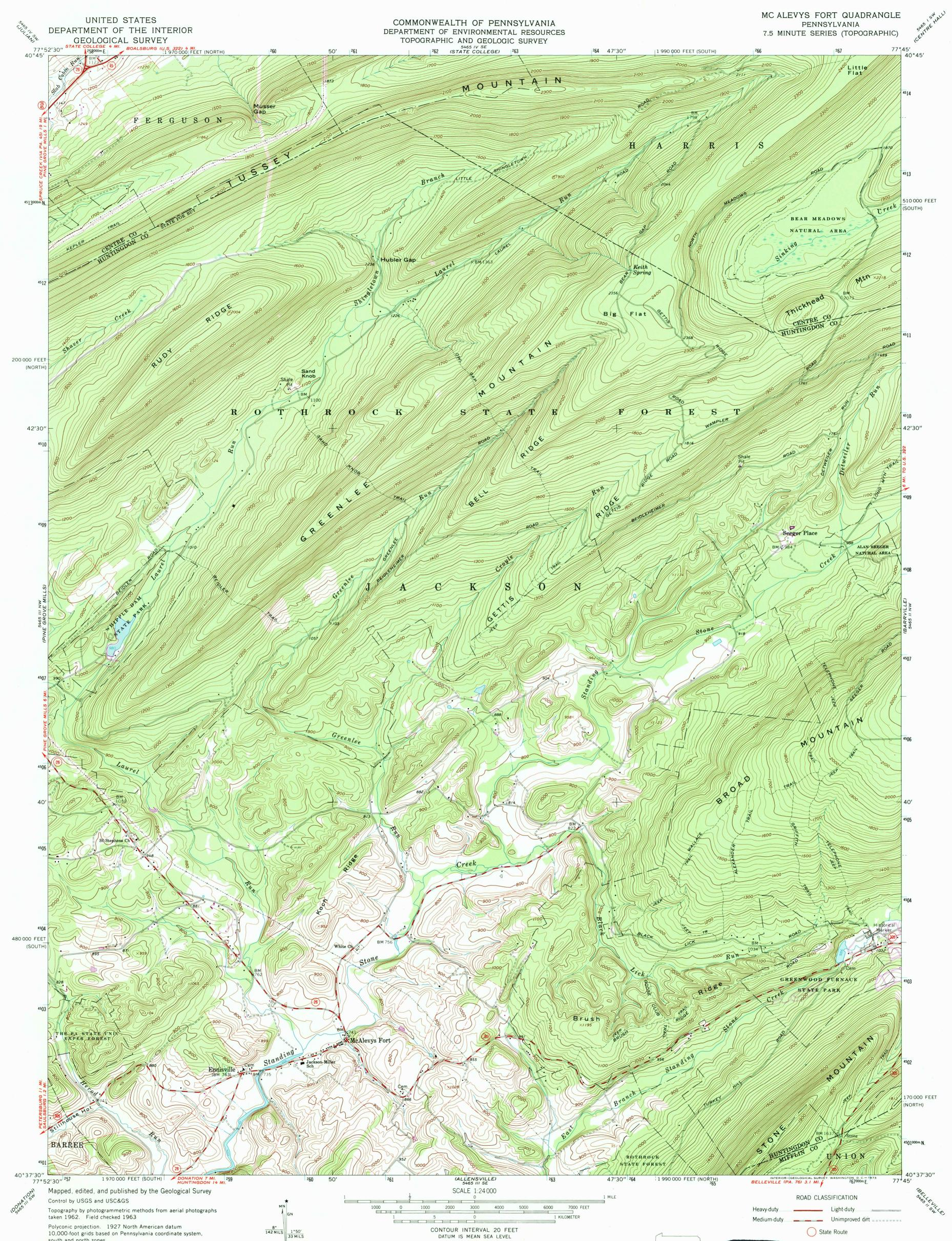
Polyconic projection. 1927 North American datum 10,000-foot grids based on Pennsylvania coordinate system, south and north zones 1000-meter Universal Transverse Mercator grid ticks, zone 18, shown in blue
