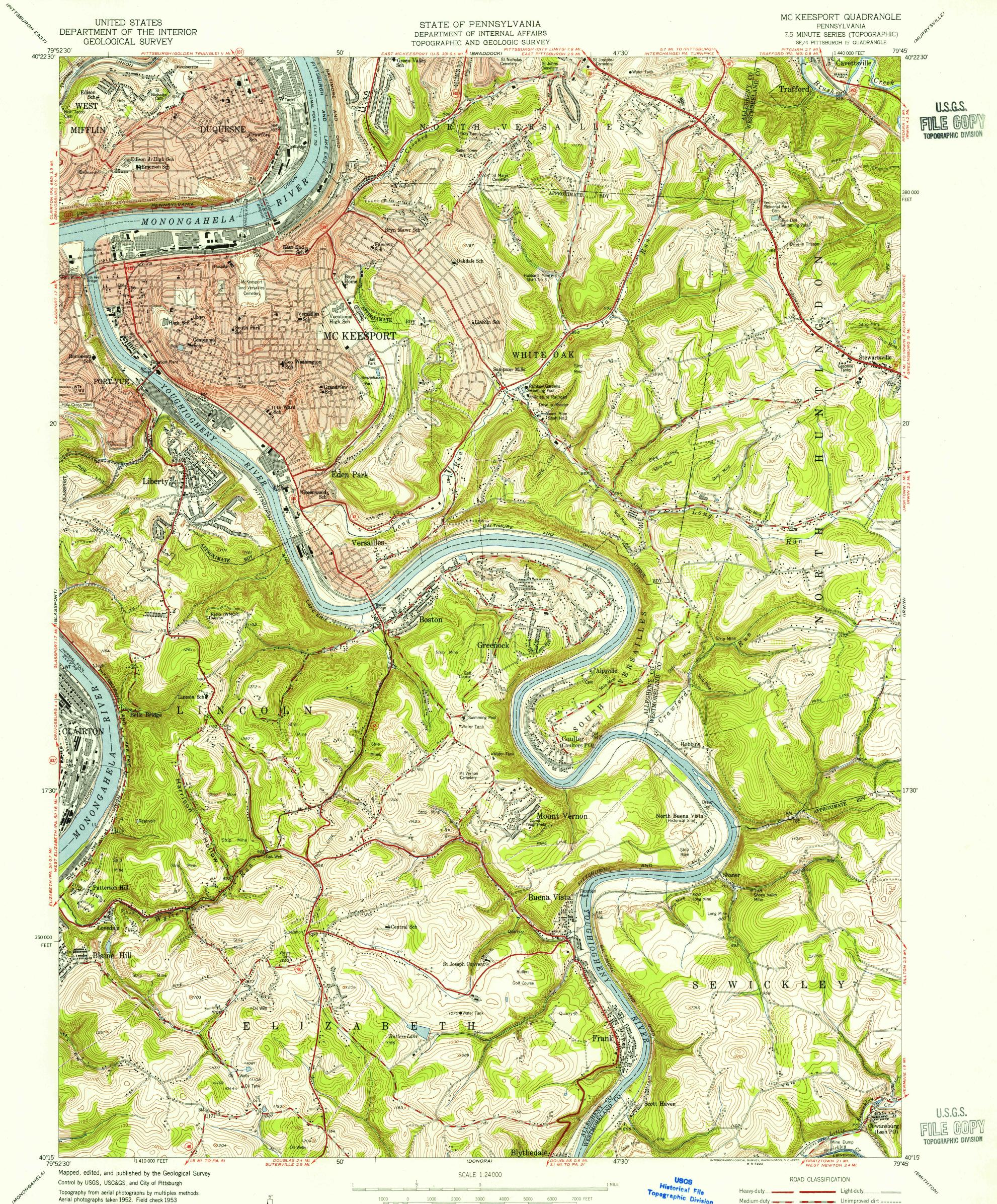
Polyconic projection. 1927 North American datum 10,000-foot grid based on Pennsylvania coordinate system, south zone Red tint indicates areas in which only landmark buildings are shown Contours in strip mine and mine dump areas compiled from 1952 photography
