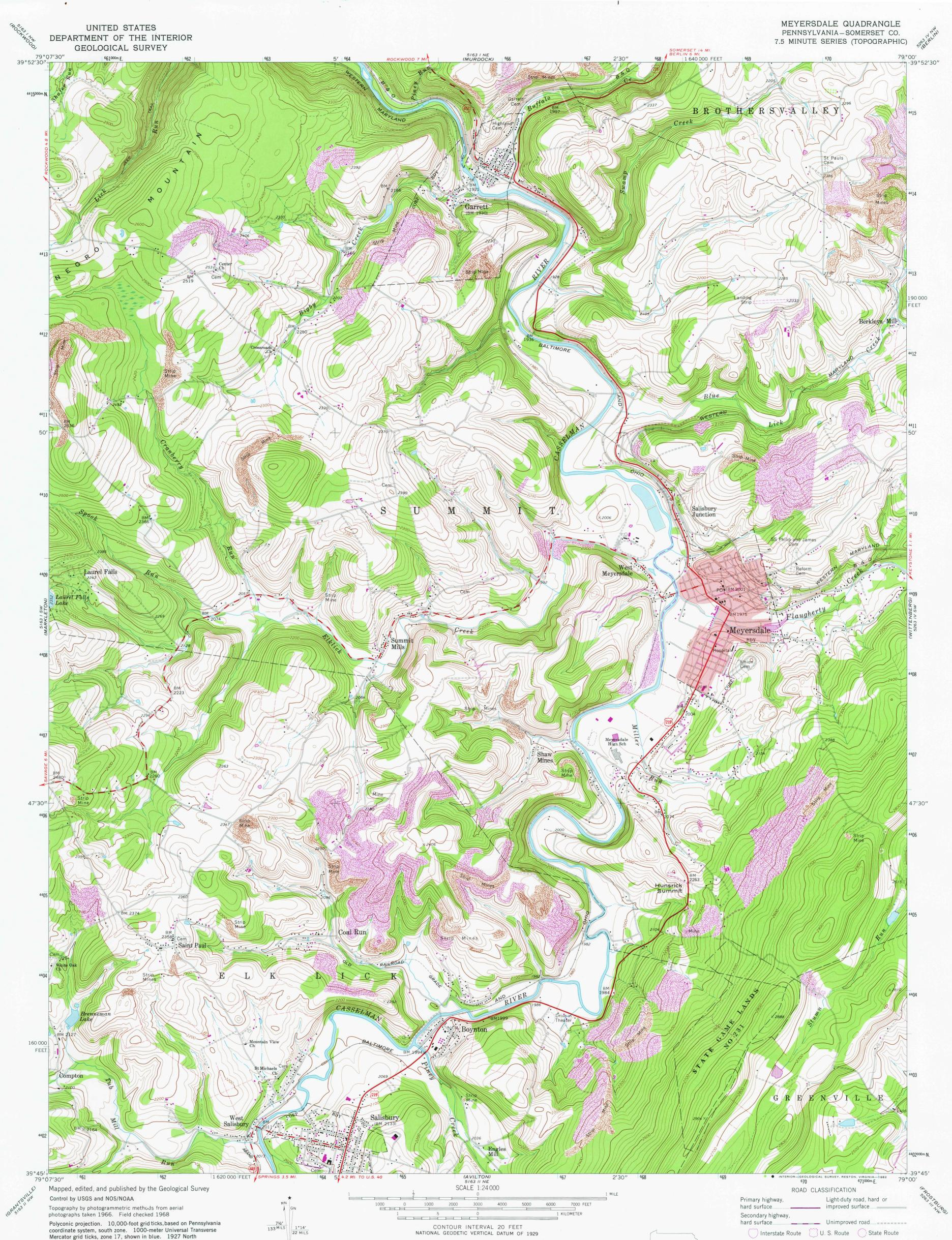
Polyconic projection. 10,000-foot grid ticks, based on Pennsylvania coordinate system, south zone. 1000-meter Universal Transverse Mercator grid ticks, zone 17, shown in blue. 1927 North American Datum. To place on the predicted North American Datum 1983 move the projection lines 6 meters south and 21 meters west as shown by dashed corner ticks
