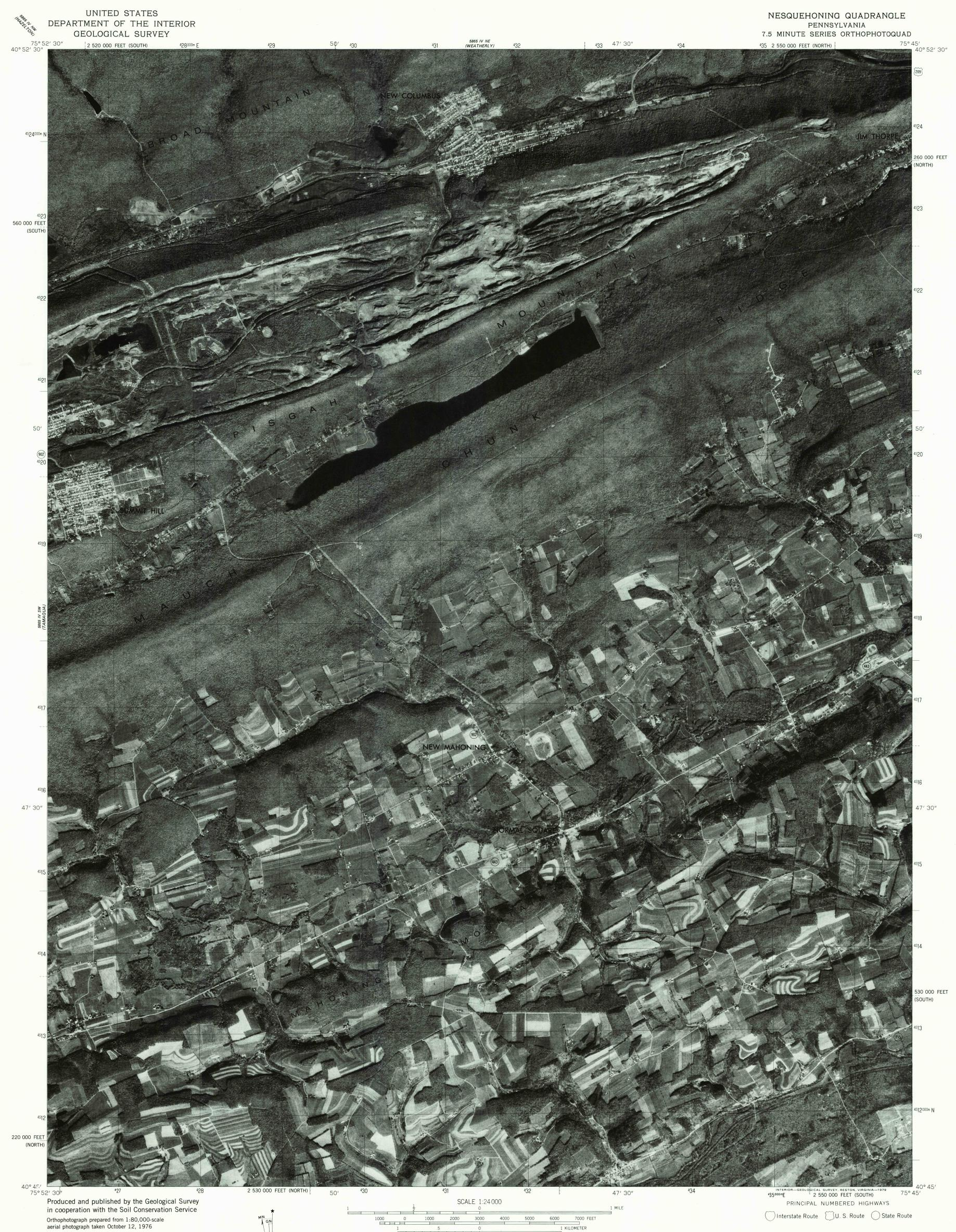
Projection: Pennsylvania coordinate system, north zone (Lambert conformal conic) 10,000-foot grid ticks based on Pennsylvania coordinate system, north and south zones 1000-meter Universal Transverse Mercator grid, zone 18. 1927 North American datum
